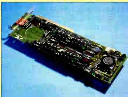
on the MPC601. A 50-MHz version of the board is available. Operating-system hooks allow the processor to write I/O to the host computer's disk or screen. This setup lets you use your host computer to write, compile, and link C programs on the MPC601. The GNU C compiler was used to compile
