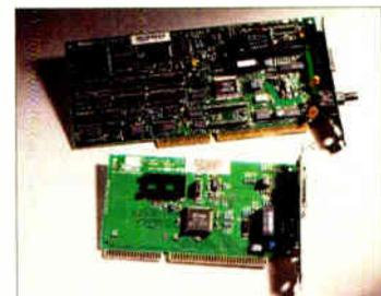
NICs built from one or two chips (bottom) allow for smaller physical designs with no performance change.
