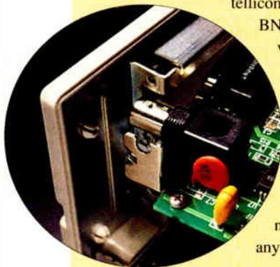
Compaq Deskpro 4/66i to insert the card for testing. Although this was the worst case, we found similar problems with other cards—BNC connectors were too high or too low. If your system is tightly packed, you may not be able to connect the BNC T-adaptor at all.
