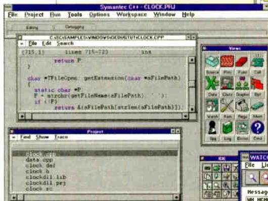
◀ **Symantec C/C++ 6.0** is a strong newcomer to the Windows C++ field. Its IDE is built around a workspace paradigm and incorporates tear-off tool palettes. Here, the current workspace is "Editing," but the "Debugging" workspace is instantly available by clicking the folder tab near the topmost menu bar.
