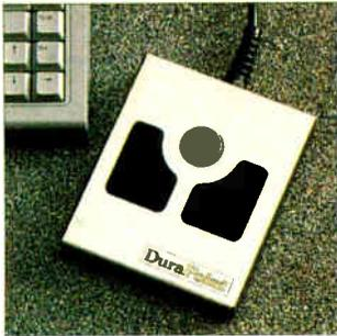
sealed against liquids, dirt, and dust. Compatible with DOS, Windows, and OS/2, the unit includes serial and PS/2 mouseport interfaces.
