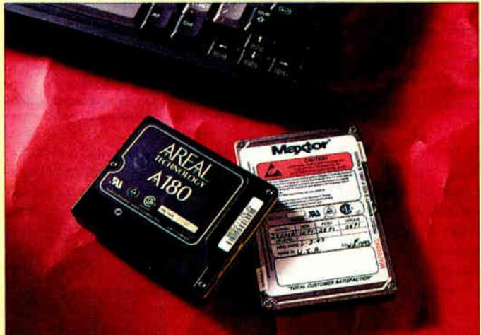
The glass platters in the Areal A180 (left) and the Maxtor 25252A drives work well with today's faster spin rates.
