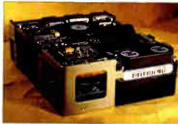
that fits more controller electronics onto the board by wrapping the flexible printed circuit board around the drive mechanics. (This same technology is often found in notebook computers.)
