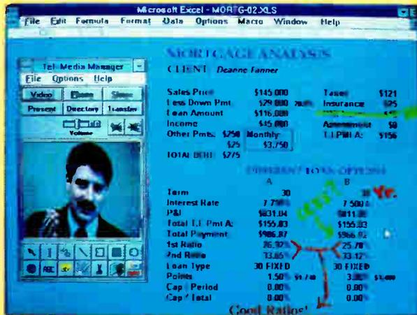
**A Cadillac among desktop video and document conferencing systems, NCR's TeleMedia Connection is a hardware and software package that supports collaborative document mark-up and real-time video-in-a-window. It uses H.261-standard compression and requires dual ISDN channels for quarter-screen video throughput of 15 fps.**
