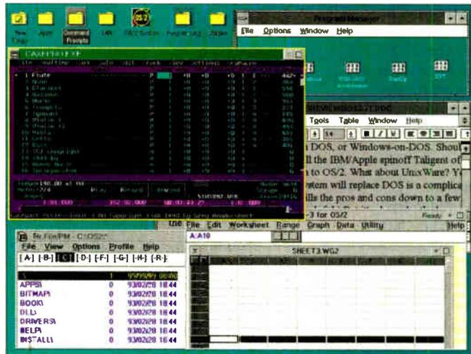
**OS/2 2.1's Workplace Shell** at a resolution of 1024 by 768 pixels and running Word for Windows, Lotus 1-2-3 for OS/2, and a few other applications. The Workplace Shell hasn't changed from version 2.0, but Windows support and device support has certainly improved. When this shot was taken, the system was simultaneously printing and playing an audio file.
