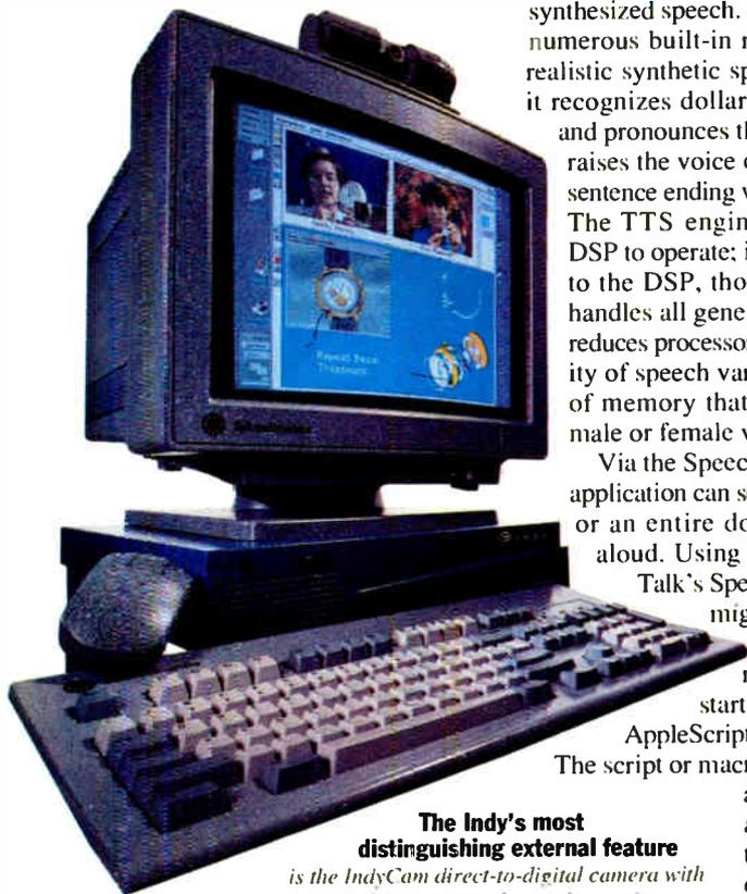
**The Indy's most distinguishing external feature** is the IndyCam direct-to-digital camera with built-in microphone, mounted atop the monitor.
