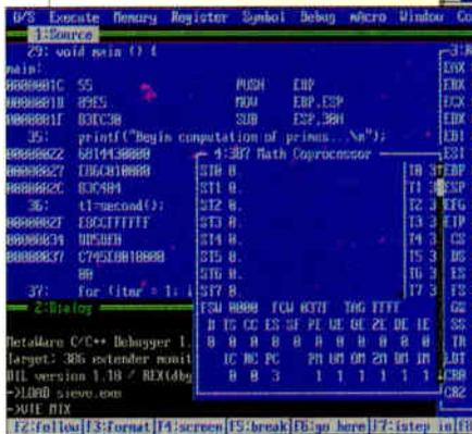
◀ **MetaWare's High C/C++** is built for speed more than comfort. MetaWare's extended-DOS debugger allows access to 32-bit flat-model executable files running under Phar Lap's DOS extender. Multiple windows allow views of C++ source code, the equivalent assembly language, and processor and coprocessor registers.
