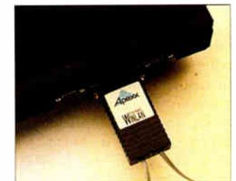
many as 250 PCs up to 600 feet away via the adapter's two RJ-11 jacks. Included are a 25-foot phone cable and a driver disk.
