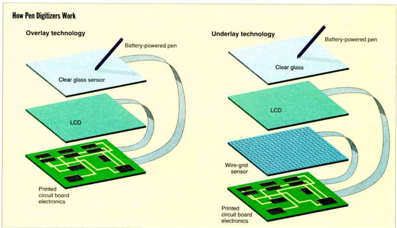
**Both overlay and underlay digitizers work similarly.** First, the pen interrupts a sensor field, sending an analog signal of the x, y coordinates to the system. The system translates the signal from analog to digital and lights the appropriate pixel.
