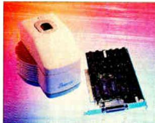
Startek's fingerprint identification system connects to a PC through the AT-bus card. The red LED fingerprint reader is at the top left.
