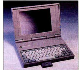
an 80- or 170-MB hard drive, an integrated trackball, and a PCMCIA Type III slot.
