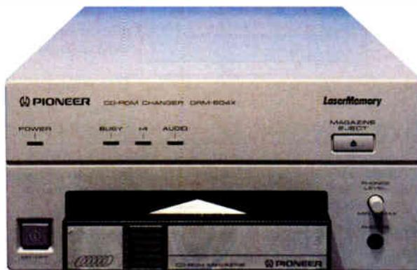
Pioneer's DRM-604X, featuring its exclusive *Quadraspin* technology, has jumped past double speed drives to a new transfer rate of over 600 KB/sec. That's four times the speed of standard drives and twice the transfer rate of double speed drives.
