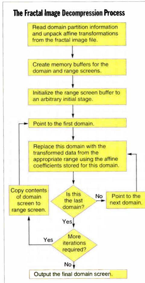
The algorithm to decompress an image stored as fractal-transform data.
