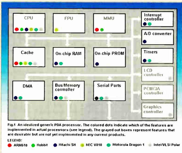
Fig. 1 An idealized generic PDA processor. The colored dots indicate which of the features are implemented in actual processors (see legend). The grayed out boxes represent features that are desirable but are not yet implemented in any current products.
