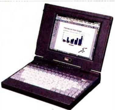
communication modules that support LANs and WANs (wide-area networks), including wireless cellular data. With an AudioDrive multimedia chip, the Inex Technologies (Santa Clara, CA) notebooks provide the means for audio presentations, vocal script, and voice E-mail. The units support up to 20 MB of main memory and up to 200 MB of storage on the removable hard drives. The LCD screen is also upgradable.
