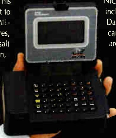
The BADGER GT-110 can be powered by a standard 9-volt alkaline or lithium battery, three 2/3A lithium batteries or a NICAD rechargeable battery pack. Built-in utilities include GT Shell, Communications, Text Editor, Data Base and Forms Manager. Application software can be downloaded from any DOS PC and data files are easily exchanged.
