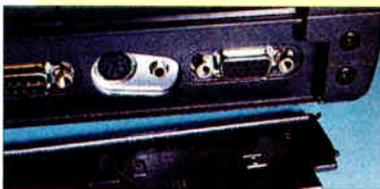
**Snap! Flimsy hinge pins** on the Compaq Contura's port-cover plate break off with the slightest provocation. Thicker pins proved sturdier, but the best solution was the Toshiba Satellite's, with sliding doors covering its ports. Note that this problem is not restricted to Compaq; other vendors, including Twinhead and Texas Instruments, are equally guilty.
