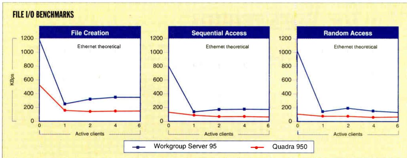
File I/O benchmarks for the Workgroup Server 95 and the Quadra 950. The Workgroup Server had a 500-MB hard drive and 16 MB of RAM to the Quadra's 230-MB hard drive and 12 MB of RAM. The figure shows aggregate network throughput while creating files and during sequential and random access. The Workgroup Server maintains a high network throughput at up to six highly active clients, although, of course, still well below theoretical Ethernet bandwidth.
