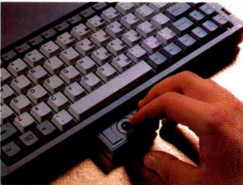
The integrated track ball slides out from a compartment by the space bar on the keyboard. You simply pull it out and go to work. Finished? Just slide the track ball back into the ColorBook.
