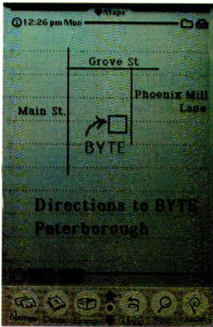
The MessagePad features a row of "hard icons" at the bottom of the screen that provide access to frequently used functions.
