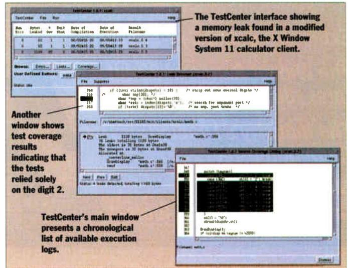
The TestCenter interface showing a memory leak found in a modified version of xcalc, the X Window System 11 calculator client.
