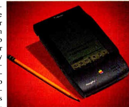
**Apple's MessagePad** is promised to be the first in a family of products based on the Newton architecture. Newton licensees are planning to introduce everything from smart telephones and fax machines to advanced cable TV converters.
