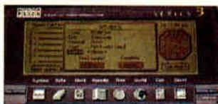
Instead of the Series 3's screen that displays 40 columns and nine rows (middle photo), the Series 3a (bottom and top photos) offers an 80-column, 18-row display.
