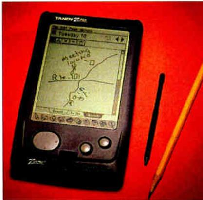
**Tandy and Casio** collaborated on the Zoomer, a PDA that strongly resembles the Apple MessagePad but is built on a completely different hardware and software architecture.
