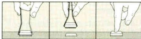
*Talk about immediate gratification. Just use the chip removal tool provided to pull out your 386DX chip (16, 20, and 25 MHz versions only at the moment), and plug our Cyrix Upgrade Microprocessor into the empty socket. Then get ready for screaming 486 power.*
