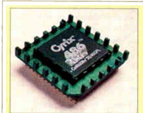
When installing Cyrix's Cx486DRx2 upgrade, I found that the hardest part of the task is pulling the old processor out of the system's motherboard. Once that was accomplished, installation was fairly easy. Cyrix supplies a chip puller (which resembles a shoehorn) that makes the job easier.
