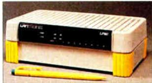
and eight ports, respectively, that let you connect up to eight nodes on an existing network via a single transceiver. In stand-alone mode, the LPMs let you set up a two-, four-, or eight-node LAN.
