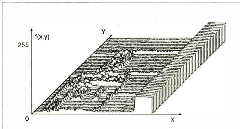
A 2-D gray-scale image actually has three dimensions: height, width, and intensity. This is evident in the above graph.
