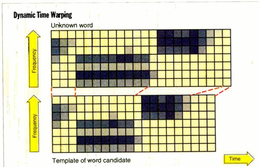
**When an unknown word is spoken,** it is compared to stored templates (i.e., frequency time pictures) of each word to get the best match. Dynamic time warping allows a match to be made so that the best-matching parts of each word align, making the match less sensitive to the speed of speaking.
