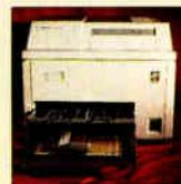
We could distinguish the output of the Tektronix Phaser IISDX from a photograph, but of all the printers we reviewed, the Phaser IISDX produces the most photograph-like output. Its dye-sublimation print engine blends inks together to produce areas of true color. No dither patterns were visible, raising the Phaser IISDX above any other non-dye-sublimation printer. It placed fine lines nearly perfectly, without gaps and with blending that was visible only with the aid of a microscope.
