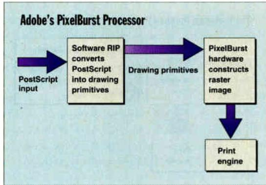
**The Adobe PixelBurst processor** can significantly boost the processing speed of raster files. It uses the list of drawing primitives produced by the software RIP to construct the raster image sent to the printer.
