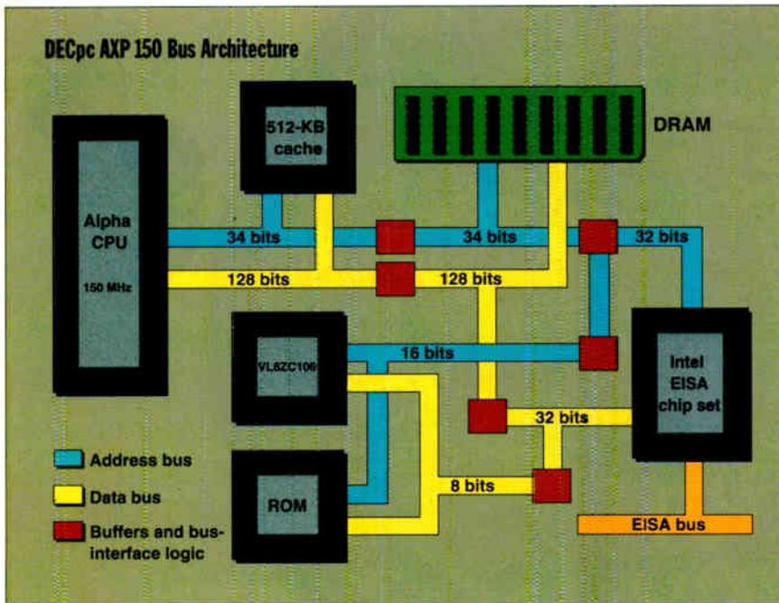
**A simplified block diagram of the DECpc AXP 150.** The buffers and interface-logic components have the tricky job of connecting buses of different widths and carrying different signal protocols. The VL82C106 chip is a one-chip source of fundamental I/O devices (i.e., serial ports, a parallel port, and keyboard and mouse interfaces).
