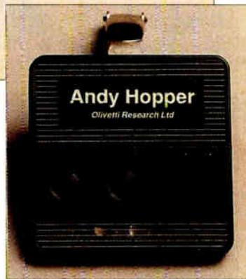
and easy maintenance) and have a very simple user interface. ORL's Active Badge is a plastic box some 2 inches square by 1/4 inch deep (55 by 55 by 7 mm) weighing 1.4 ounces (40 gm). Its only external control is a test button.
