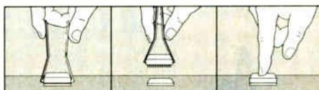
*Here's how to get an instant 486. Just use the chip removal tool provided to pull out your 386DX chip (16, 20, and 25 MHz versions), and plug our Cyrix Upgrade Microprocessor into the empty socket. Installing the SX version is even easier. It just clips on over the existing chip.*
