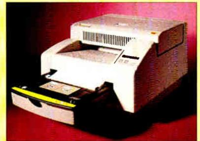
For computer connections, the ColorEase offers a Centronics parallel port, a DB-9 RS-232 serial port, and a mini-DIN-8 LocalTalk port. Two 50-pin high-density SCSI connectors let you attach an external SCSI hard drive. An Ethernet interface board is optional. Windows and Mac drivers are available.
