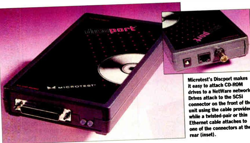
Microtest's Discport makes it easy to attach CD-ROM drives to a NetWare network. Drives attach to the SCSI connector on the front of the unit using the cable provided, while a twisted-pair or thin Ethernet cable attaches to one of the connectors at the rear (inset).
