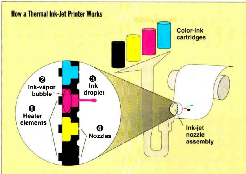
Thermal ink-jet printers use heat ① to create a vapor bubble ② that forces a droplet of ink ③ through a nozzle ④.
