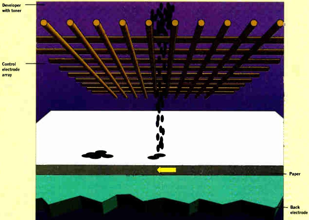
**Array's TonerJet by Array technology** places an electrically charged control electrode array, which can be either a wire mesh or a perforated flexible printed circuit board, between the toner and the paper. A back electrode beneath the paper attracts toner and pulls it through the holes in the control electrode array. The toner lands on the paper and forms a dot.
