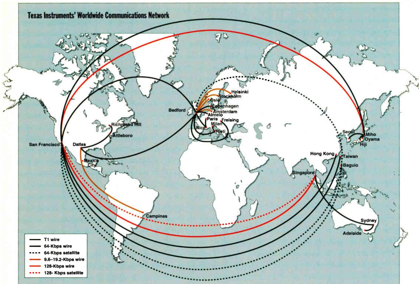
Texas Instruments' global communications network illustrates just how complex worldwide networking can get. The LAN internetwork spans several different transmission methods, from dedicated modem lines to satellite links.
