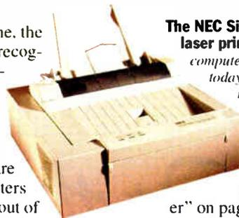
**The NEC Silentwriter Superscript 610 laser printer** is designed to use the computer's processor and memory. With today's faster processors, this feature reduces the cost of the printer, without degrading system performance for most users.
