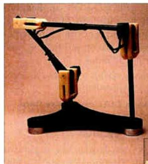
gers like a pencil to convey spatial position (x, y, and z) and orientation information (roll, pitch, and yaw) to the host processor. From Immersion Human Interface (Palo Alto, CA), the device is self-calibrating with sen-
