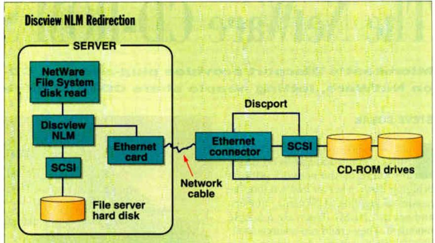
The Discport attaches as a network node, but CD-ROM drives attached to it appear logically attached to a server due to Microtest's NLM. The NLM on the server reroutes CD-ROM accesses directed at the server to the Discport, which translates between Ethernet packets and SCSI-2 blocks.
