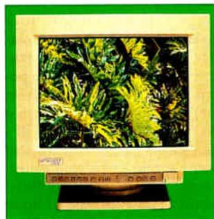
monitor has a horizontal frequency scan rate of 30 to 65 kHz that supports noninterlaced resolutions of up to 1280 by 1024 pixels; its 1024- by 768-pixel resolution has a 76-Hz refresh rate. The 2000DC is VESA DPMS compliant and meets Energy Star guidelines.
