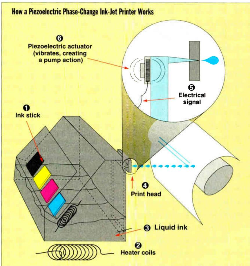
Piezoelectric phase-change ink-jet printers use a solid ink ①. A heating element ② melts that ink ③, which then goes to the actuator in the print head ④. Pulses of electricity ⑤ create a pumping action in the actuator ⑥, and this forces the ink out onto the paper. The ink then solidifies as soon as it touches the paper, avoiding the spreading, or wicking, problems associated with liquid inks.
