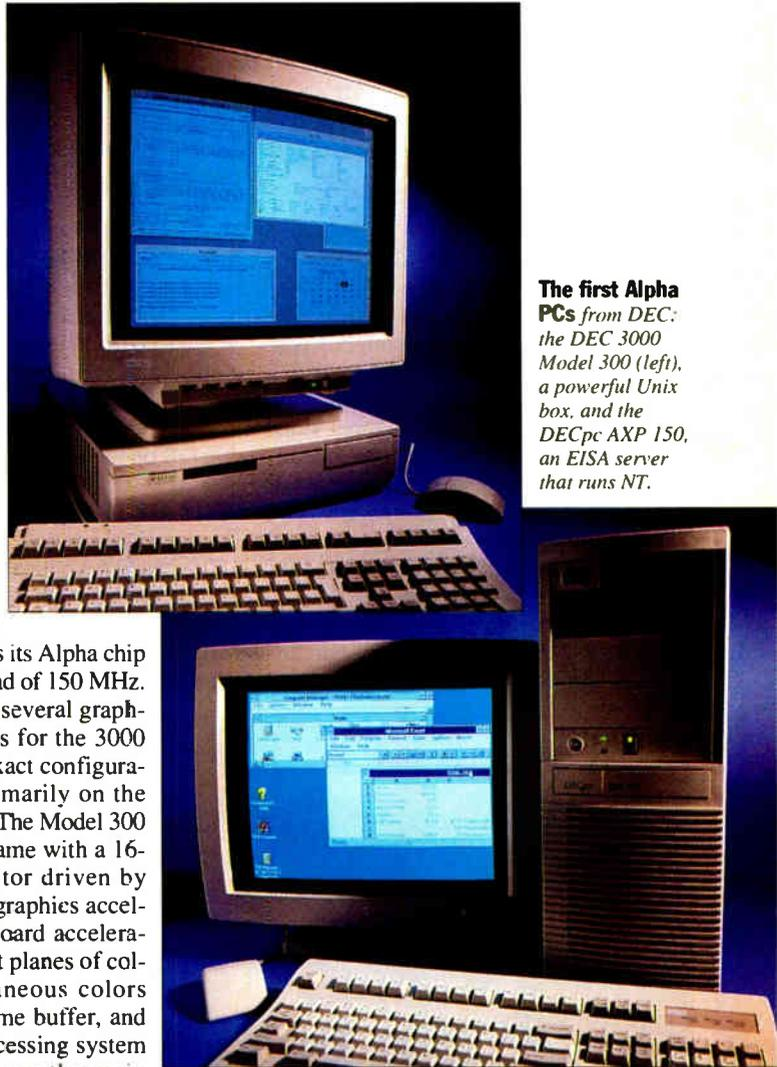
**The first Alpha PCs from DEC:** the DEC 3000 Model 300 (left), a powerful Unix box, and the DECpc AXP 150, an EISA server that runs NT.
