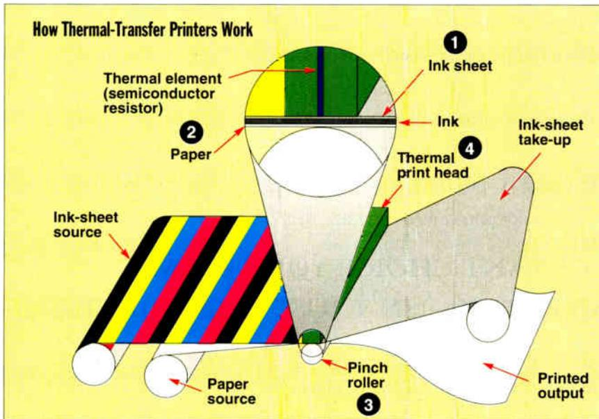
Thermal-transfer printers use a banded, multicolor ink sheet ① that rolls simultaneously with the paper ② toward a pinch roller ③. This squeezes them together toward the thermal print head ④. Commands from the computer or printer turn tiny semiconductor resistors in the print head on or off to melt or resolidify the ink onto the paper. After each pass, the ink sheet advances to the next color band and the paper retracts to its starting position until the full-color printing process is complete.
