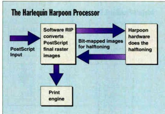
**The Harlequin ScriptWorks RIP** works hand in hand with the Harpoon processor to increase the throughput and enhance the image of PostScript files. The Harpoon processor deals only with the halftoning process.
