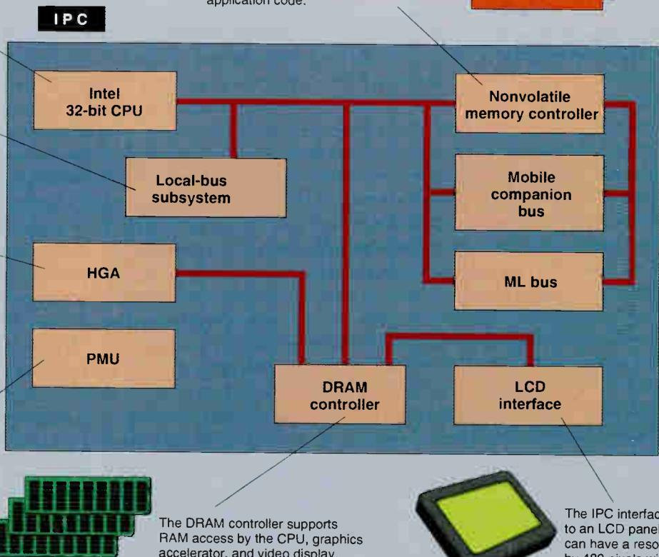
**The Polar chip set** is a highly integrated solution that offers just about all the functionality you need in a PDA system.
