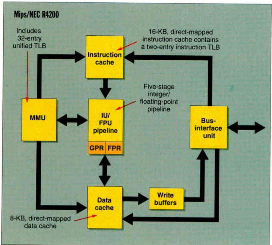
**The R4200** integrates a complete RISC pipeline and 24-KB cache on a die 82 mm<sup>2</sup>. Its low power consumption and high performance make it ideal for notebook systems.
