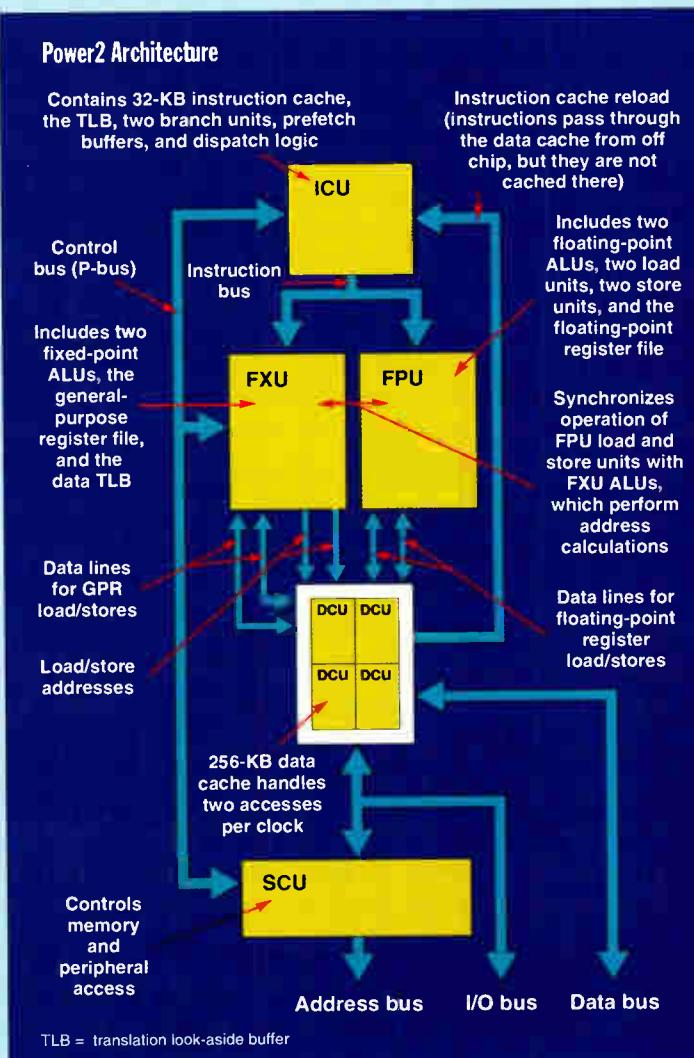
**With six separate chips** in a single multichip module, the Power2 can, under ideal conditions, issue and execute six instructions at one time.
