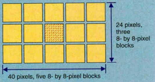
**The MPEG algorithm** searches a 40- by 24-pixel block surrounding a single 8- by 8-pixel block to find the best alignment between the reference frame and the current one.
