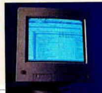
A new product from IBM's new PC Company, the 17P was the clear winner for image quality in this class. We rated it best among 17-inch monitors on the image-quality screen tests, and it proved best at the legibility and sharpness tests. Based on a Sony Trinitron tube, the 17P offers VESA-compliant power management, MPR II compliance, and a complete set of controls for adjusting the screen and color reproduction.
