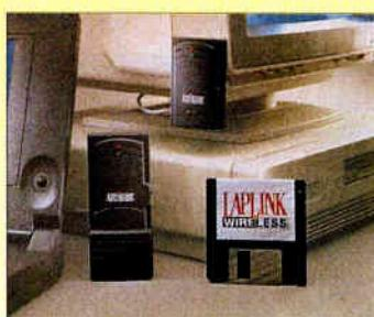
*LapLink Wireless with AirShare, which has a range of about 30 feet indoors, lets two computers automatically synchronize and share files using a wireless radio connection.*
