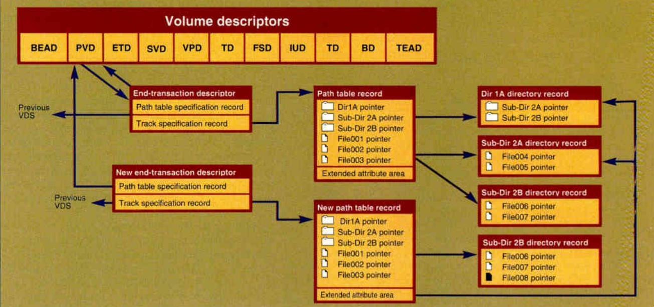
A CD-WO structure, illustrating the arrangement of a set of directories, subdirectories, and files, with a new file (File008) added.
