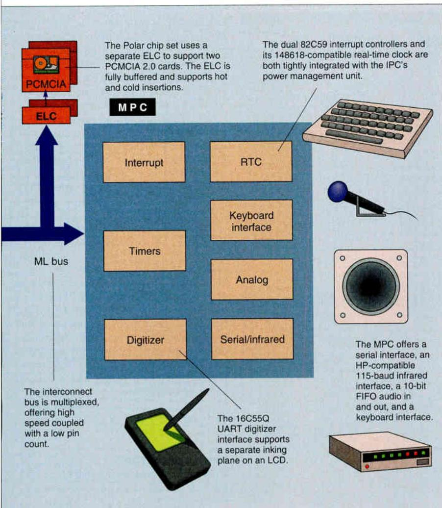
process and supports 3.3- and 5-V operation. The IPC uses a fully static core that can preserve the state of the CPU even when the system clock is shut down. The IPC can generate 20-, 25-, or 33-MHz system clocks.
