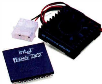
It's a fact. 486 chips run hot, often exceeding 185°F! Now, you can cool your 486 to a safe 85°-95°F with our popular CPU-Cool. It prevents random system errors and other heat-related problems. Consists of a mini-fan embedded in a die-cast heat sink that easily mounts on the CPU. Powered by a spare drive connector. Effective, inexpensive insurance!
