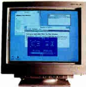
**The AcerView 76i displays settings** on the screen, which makes adjusting images for brightness, contrast, or distortion easy. It can display the settings in five languages and gives the user a numerical setting for each control.
