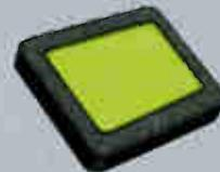
The IPC interfaces directly to an LCD panel. The panel can have a resolution of 640 by 480 pixels with 16 gray shades.
