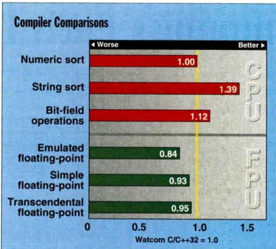
**When generating Windows NT executable files, the compiler in Microsoft Visual C++ 32-bit Edition performed equivalently to Watcom C/C++'s compiler, the fastest one we've tested. Microsoft scores are indexed against Watcom results, which equal 1. The tests consisted of BYTE's portable C benchmarks, with both compilers set to generate speed-optimized 486 code. Tests ran on a 50-MHz Everex 486DX2 with 256 KB of cache and 16 MB of RAM.**
