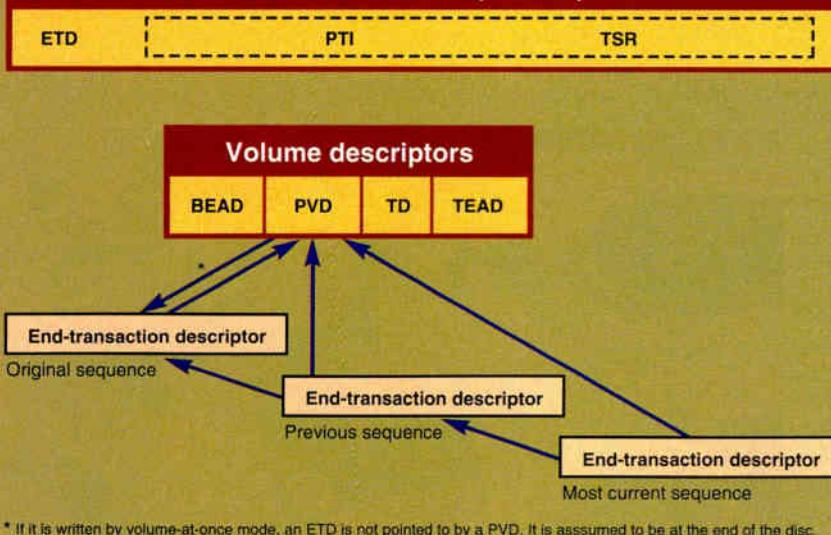
The structure of an ETD and how ETDs are linked when material on the disc is updated.
