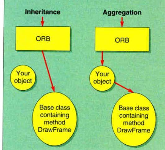
**In both cases**, your object passes on calls to draw its frame to a method called *DrawFrame*. In the SOM inheritance model, the ORB (object request broker) vectors the *DrawFrame* call directly to the base class object where it is implemented. In the COM aggregation model, your object must add to its vtable the necessary pointer to the *DrawFrame* method in the base class object.
