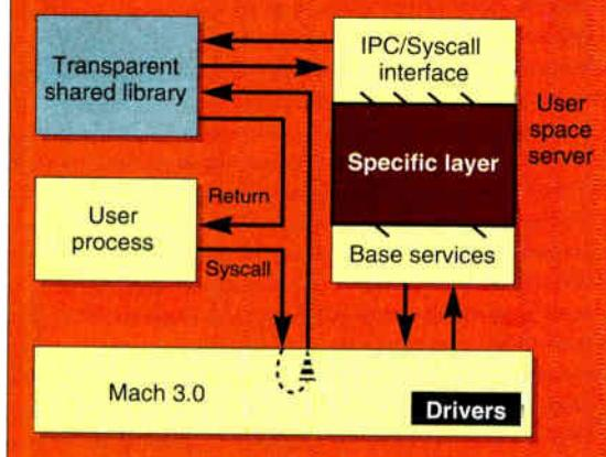
**OSF/1 1.3 runs the OSF/1 server as a monolithic component on top of the Mach microkernel.**
