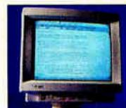
KFC packs quite a lot into this \$495 product. The 15-inch CA1507 offers resolutions as high as 1280 by 1024 pixels at 60 Hz noninterlaced. The trade-off for low cost is only average quality scores. The monitor provides a full set of image-adjustment controls, including pincushion, image rotation, and power management. It uses the VESA DPMS power management control signals to meet Energy Star requirements.
