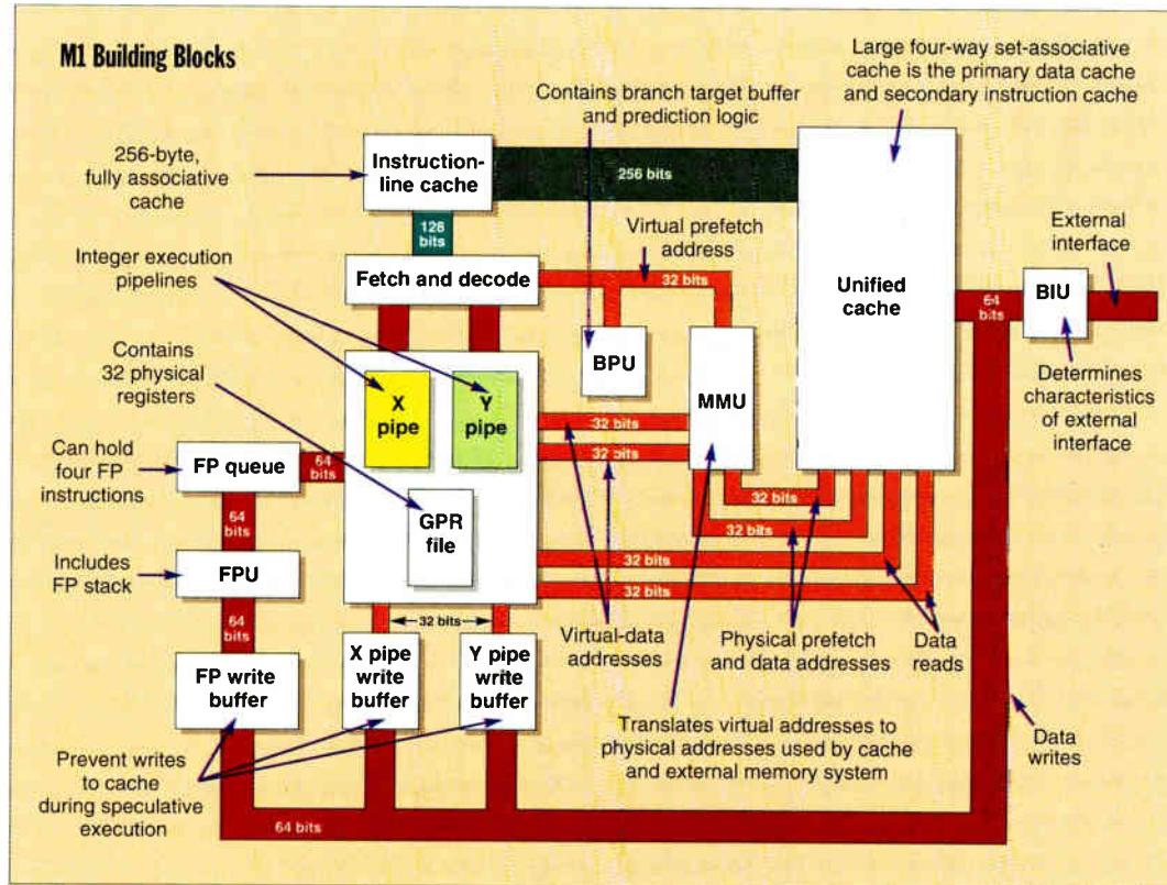
Like the Pentium, the M1 features dual-integer pipes. Unlike the Pentium, the M1 uses a unified cache in conjunction with a separate instruction-line cache. Also, the FPU on the M1 is not as aggressively pipelined as that of the Pentium.
