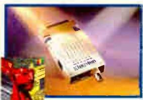
Kingston Technology's EtherRx Adapter includes both BNC (10BaseT) and RJ-45 (10Base-T) connectors which allow a laptop or notebook PC to access a LAN via the PC's parallel port.
