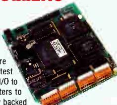
Use our Little Giant™ and Tiny Giant™ miniature controllers to computerize your product, plant or test department. Features built-in power supply, digital I/O to 48+ lines, serial I/O (RS232 / RS485), A/D converters to 20 bits, solenoid drivers, time of day clock, battery backed memory, watchdog, field wiring connectors, up to 8 X 40 LCD with graphics, and more! Our \$195 interactive Dynamic C™ makes serious software development easy. You're only one phone call away from a total solution.
