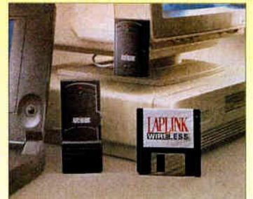
*LapLink Wireless with AirShare, which has a range of about 30 feet indoors, lets two computers automatically synchronize and share files using a wireless radio connection.*
