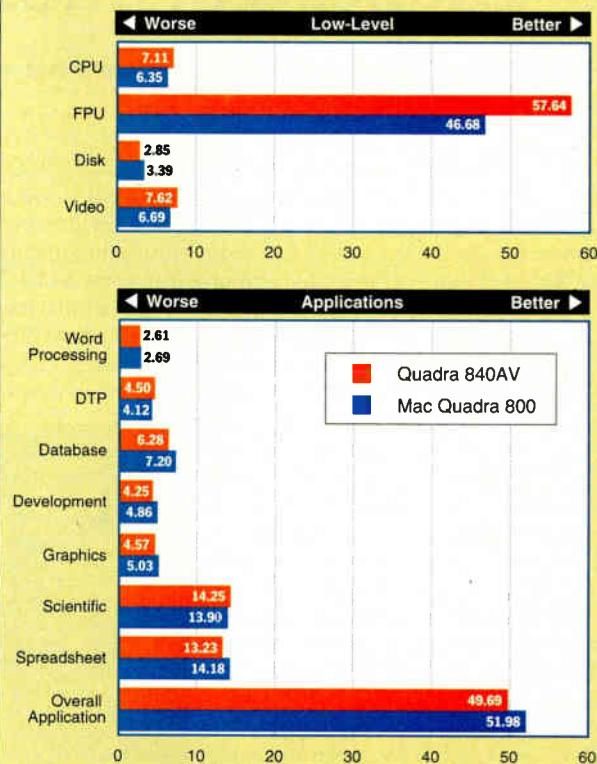
Results are indexed. For each individual test, a Mac Classic II=1.0; for the Overall Application Index, a Classic II=7.0. The Classic II used 512- by 342-pixel screens; the Quadras used 640 by 480 pixels. For the 68040-based Macs, caches were disabled only for Word Processing tests, and PageMaker 4.2 was used for DTP tests.
