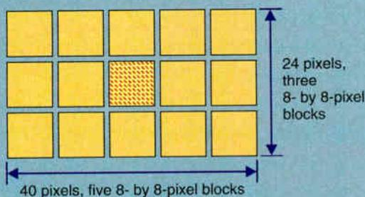
**The MPEG algorithm** searches a 40- by 24-pixel block surrounding a single 8- by 8-pixel block to find the best alignment between the reference frame and the current one.
