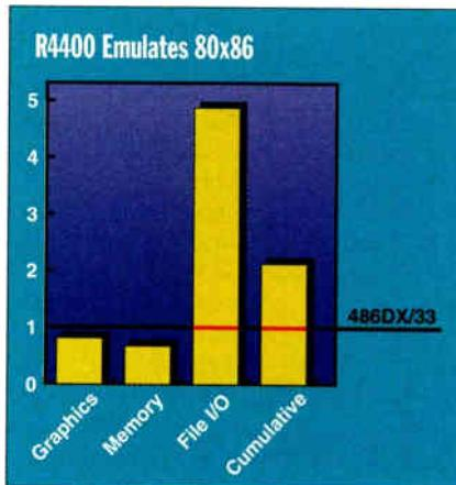
**Running the BYTE low-level Windows benchmarks, an SGI Magnum 7SSC (Mips R4400 processor) turns in a credible performance in emulation mode against an IBM PS/2 Model 90 XP 486 (486DX/33 processor). The cumulative index is skewed by the fantastic performance of the Windows NT file system.**
