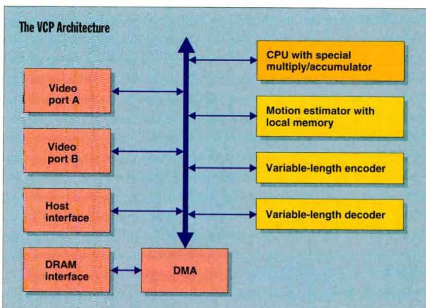
**Although the CPU controls the chip,** it is the motion estimator, the memory subsystem, and the variable-length encoders that provide most of the chip's computational power.
