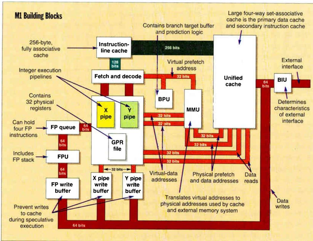
**Like the Pentium**, the M1 features dual-integer pipes. Unlike the Pentium, the M1 uses a unified cache in conjunction with a separate instruction-line cache. Also, the FPU on the M1 is not as aggressively pipelined as that of the Pentium.
