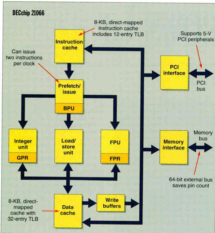
**Integrating an Alpha core** with both memory and PCI controllers yields a powerful chip that is easy and inexpensive to integrate into a system. Despite its added functionality, the DECchip 21066 requires 144 fewer pins than the 21064.
