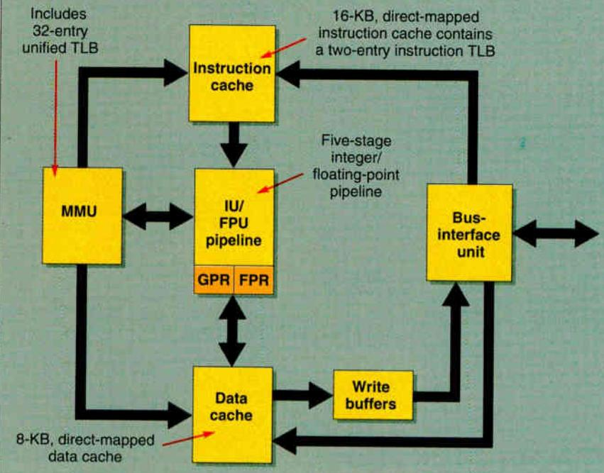
The R4200 integrates a complete RISC pipeline and 24-KB cache on a die 82 mm<sup>2</sup>. Its low power consumption and high performance make it ideal for notebook systems.
