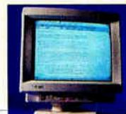
KFC packs quite a lot into this \$495 product. The 15-inch CA1507 offers resolutions as high as 1280 by 1024 pixels at 60 Hz noninterlaced. The trade-off for low cost is only average quality scores. The monitor provides a full set of image-adjustment controls, including pincushion, image rotation, and power management. It uses the VESA DPMS power management control signals to meet Energy Star requirements.
