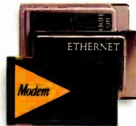
**Two separate PCMCIA slots:** A 16mm and a 5mm slot are your keys to expansion, now and into the future—for modems, storage and more.
