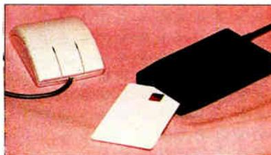
(\$395) operates in Windows 3.1 and works independently of your network software. A chip on the card stores information that lets you access your passwords; you activate the card via a PIN. The card encrypts files via DES with a separate key that's randomly generated for each file. In addition to storing private information, you can store information that's open to public view.
