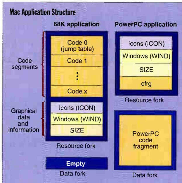
**The structure of a 68K Mac application and a PowerPC Mac application.** The program code for the PowerPC Mac (i.e., the code fragments) is located in the data fork of the file, while resources for windows, icons, and controls still reside in the resource fork.
