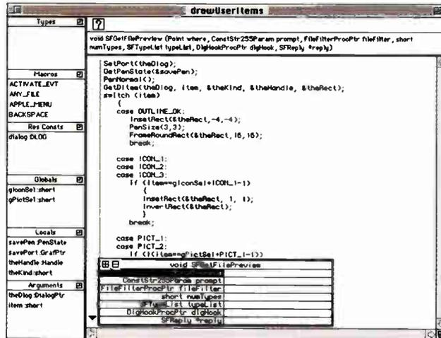
**VIP-C templates** provide easy reference to the parameters for infrequently used functions. The window at the top holds a routine prototype, and the bottom window holds a template for that routine, ready to be filled in.
