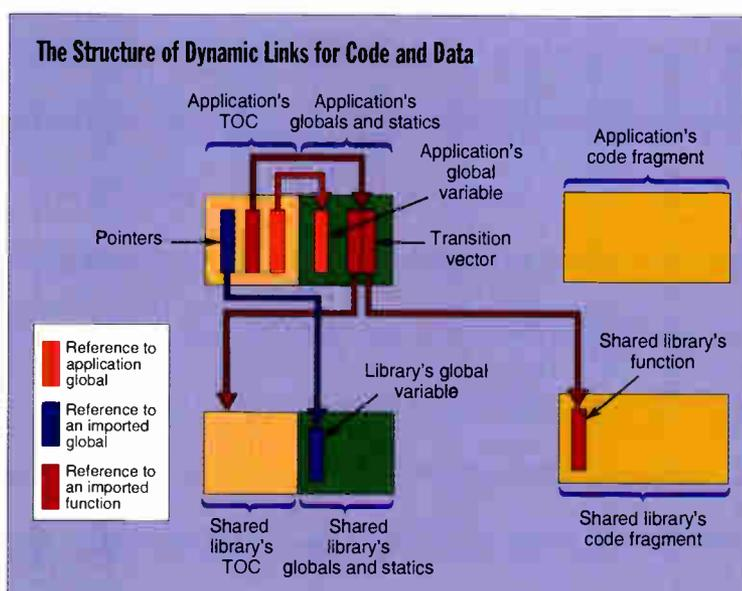
**A PowerPC application** uses a TOC to point to various structures required by the application. The TOC points to the application's own global and static variables, other fragments' globals, and transition vectors that point to the TOC and function-entry points of shared libraries that the application uses.
