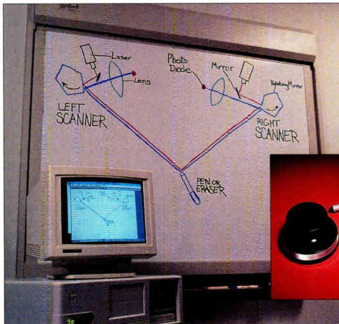
Each of the SoftBoard's pens has a specially encoded reflective collar so the laser can identify the pen and determine its color. The larger eraser uses a similar reflective surface.
