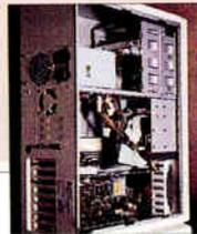
The MicroFlex-VE/66 is a roomy tower with a total of six 32-bit slots and two VL-Bus slots. There are 16 SIMM sockets that are conveniently placed on the motherboard away from the adapter slots, so you can easily upgrade the system to its maximum 128 MB of RAM. The system also accommodates four 5 1/2-inch and three 3 1/2-inch mass-storage devices.
