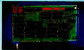
The Unicore POSTcard V2™ is a plug-in diagnostic board that monitors POST (power on self test) routines, provides continuous burn-in testing of preboot functions, and supports comprehensive system function and component diagnostics for IBM and compatible PC/XT, AT, 80386, 80486 and Pentium class machines. In addition, the POSTcard V2 has the ability to source actual IRQ usage and actually monitor DMA and IRQ lines.
