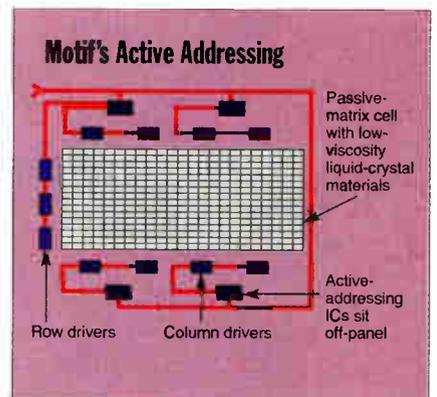
With active addressing, proprietary ASICs (application-specific ICs) that sit off the panel can address many rows simultaneously. The ASICs take the image from the graphics card and quickly calculate in real time where voltages need to be applied to the crystals. According to Motif, this technique provides near-TFT performance at a slightly higher cost than passive matrix.
