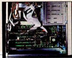
This system's large tower case holds four 5 1/4-inch and two 3 1/2-inch disk drives. Four 16-bit ISA and one VL-Bus slot are available for additional boards. The four SIMM sockets are easily accessible on the motherboard. However, a cooling fan on top of the processor obstructs access to cache memory slots. The first runner-up, American Multisystems' Info Gold 486 PCI, conveniently has its power, turbo, and reset switches in the front panel.
