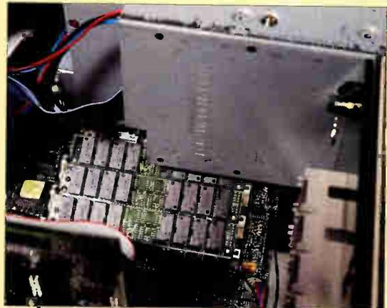
**The Acma 486 Tower includes** both a 3½-inch and 5¼-inch floppy drive. Unfortunately, the manufacturer doesn't follow the convention of designating the 3½-inch drive as the A drive. We couldn't reverse drive designations from within the BIOS setup since both drives are on the same ribbon cable connector, and the documentation did not provide any information on changing jumpers.
