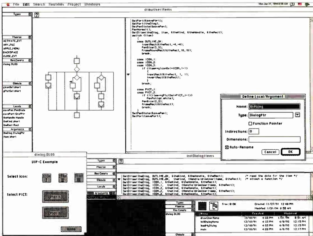
A typical VIP screen layout with an application in development. Shown are the VIP-C project window (lower right); a dialog window being designed (lower left); two routines, one in the form of a flowchart; and a local-variable definition.
