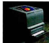
ly active ports via its resident AppleTalk, serial, and parallel interfaces. From Digital Equipment Corp. (Maynard, MA), the printer has 8 MB of memory in addition to optional EtherTalk, LAT, NetWare, and TCP/IP interfaces. RISC processing provides a printing speed of 2 pages per minute; print resolution is 300 by 600 dpi.
