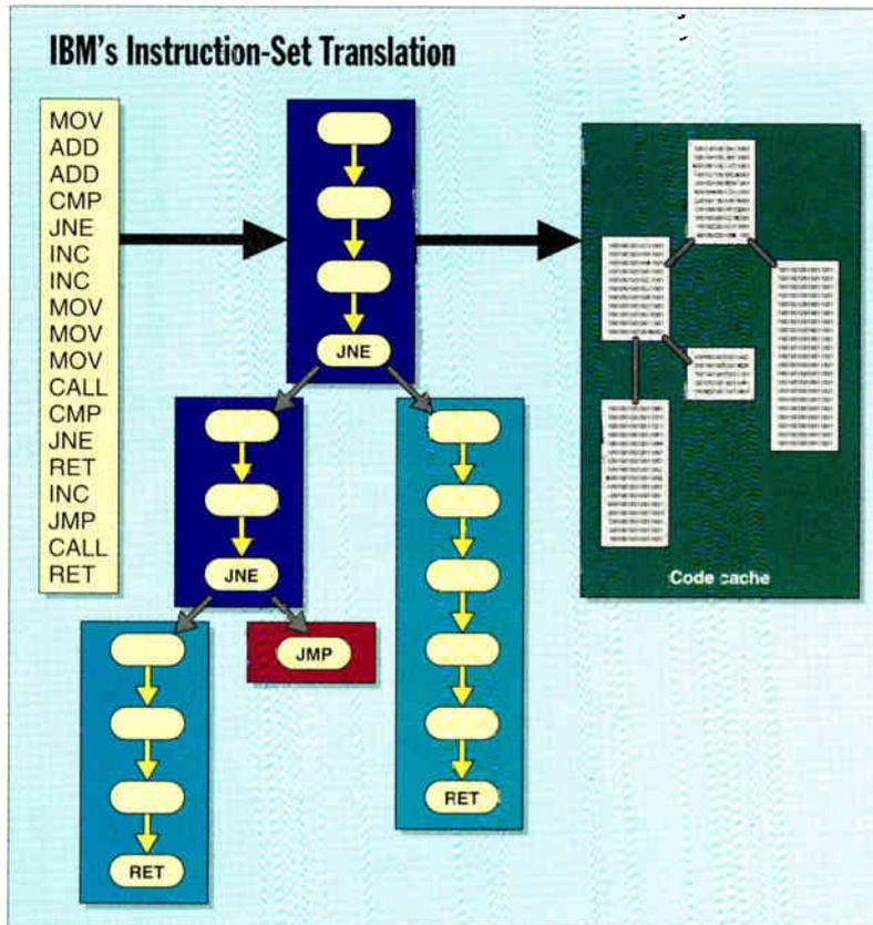
**IBM's instruction-set translation** technology works like on-the-fly compilation. The stream of Intel 80x86 instructions from the application is first analyzed and divided into logical blocks of code. Those blocks are then translated into RISC code for the host platform, "wired" together in proper sequence, and stored in a special memory cache for subsequent execution. IBM says a fast RISC-based computer can carry out all these operations without perceptible degradation of performance.
