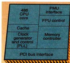
TI packs many devices into its Rio Grande chip set, but perhaps the most intriguing is the Power Management Unit (PMU) interface. TI says its 486 can turn off and on between keystrokes by switching the CPU off and on in 2 percent of the time required by rival active power management systems. TI hopes this feature will double a notebook PC's battery life.
