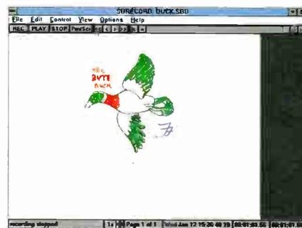
Microfield supplies software (Windows version shown) that captures the data from the SoftBoard, displays it on-screen, and saves it for future playback. The software controls simulate a VCR and allow the drawing to be played back at any speed, forward or backward, and let you print the image to any Windows-compatible printer. With SBREMOTE, an optional program, you can transmit an image as it's drawn to a remote site over any high-speed asynchronous modem.
