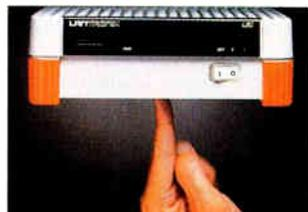
two AUI ports and a serial port for an ASCII terminal that's acting as a local management console. From Lantronix (Irvine, CA), the \$1695 unit is compatible with Telnet, DECnet, SNMP, SunNet Manager, and HP OpenView and has configuration utilities for use with AppleTalk and NetWare.
