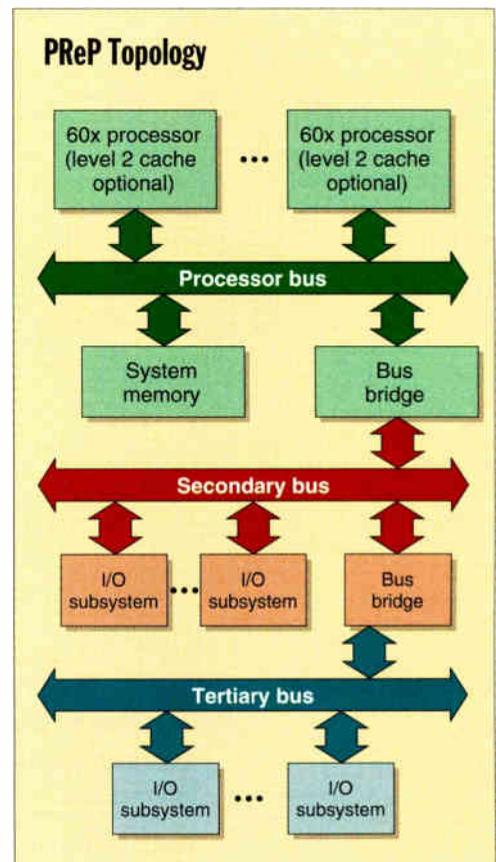
PReP systems can incorporate many different bus types into a hierarchical structure. At the top is the processor bus, which connects one or more processors and their caches to both system memory and system I/O. Connection to system I/O comes via a bus bridge to a secondary bus; in most PReP systems, this secondary bus will be PCI. The secondary bus can then bridge to a tertiary bus, such as ISA, and so on.
