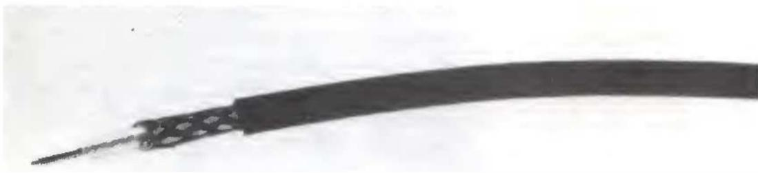
Photo 1: Coaxial cable consists of a central conductor, an outer conductive braid, and a protective coating. It is bulky and expensive, but it has good characteristics as a transmission line for data.
