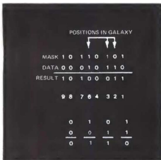
Figure 6: The EXCLUSIVE OR function of Boolean logic is used to complement bits selected according to the galaxy information stored for the position just shot.
