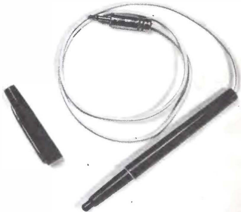
Photo 4: This shows a pen based on the TI type L-63 photocell, built using a marking pen case.
