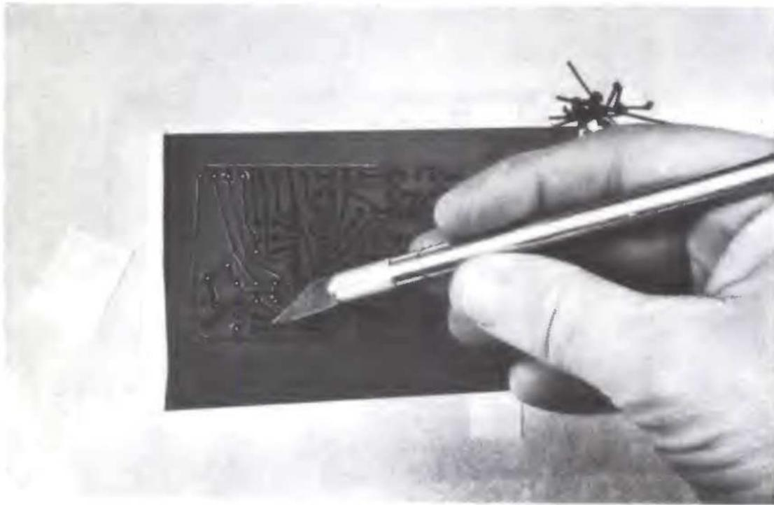
*Photo 4: The "Cut-N-Peel" Method. A sheet of red mylar film on clear acetate backing is placed over the pattern to be copied. The negative is made by carefully tracing the pattern with a razor or sharp knife, then removing the red film wherever component pads and connections are to be made. (A trade name for the film used in this method is "Rubylith.") The negative is then transferred to sensitized copper and etched.*
