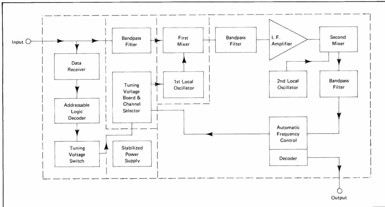
Figure 9. Oak Addresso-Code Converter/Decoder Functional Block Diagram
