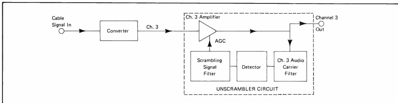
Figure 5. Oak Decoder Block Diagram
