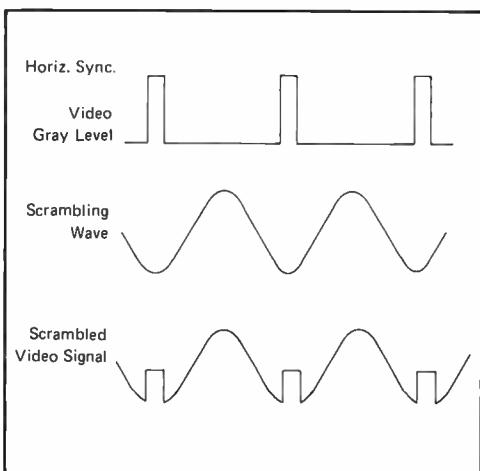
Figure 3. Scrambling Waveforms
