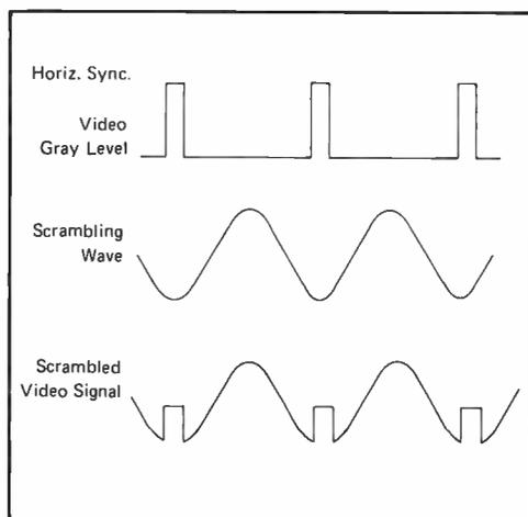
Figure 3. Scrambling Waveforms
