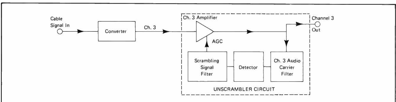
Figure 5. Oak Decoder Block Diagram
