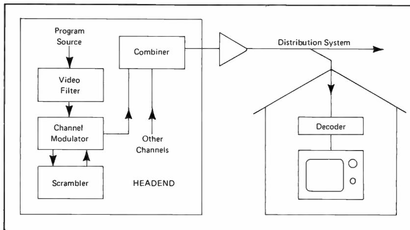
Figure 4. Oak Multi-Code System Block Diagram
