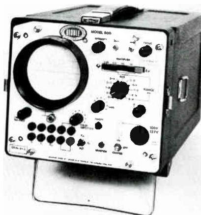
The Model 600, using the Time Domain Reflectometry Principle, has a range of 75 miles and accuracy of  $\pm 0.5\%$  of range. A single sinusoidal pulse is generated at different repetition rates depending on the size of the loading coil. High sensitivity results from a variable output to 60 volts and gain to greater than X1000. The Model 600 is fully portable and operates either from line voltage or internal rechargeable batteries, giving up to 5 hours continuous operation.
