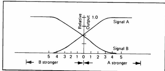
Figure 3. Typical Capture Characteristics
