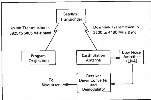
Figure 1. Satellite-Earth Station System, Block Diagram
