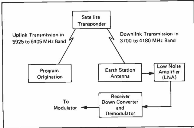
*Figure 1. Satellite-Earth Station System, Block Diagram*
