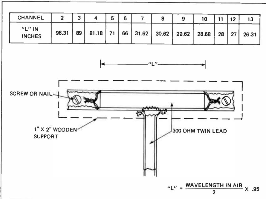
*Drawing 3. Folded Dipole Antenna*
