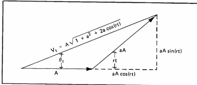
Figure 2. Discriminator Output Phasor Diagram
