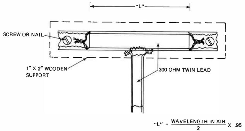
*Drawing 3. Folded Dipole Antenna*
