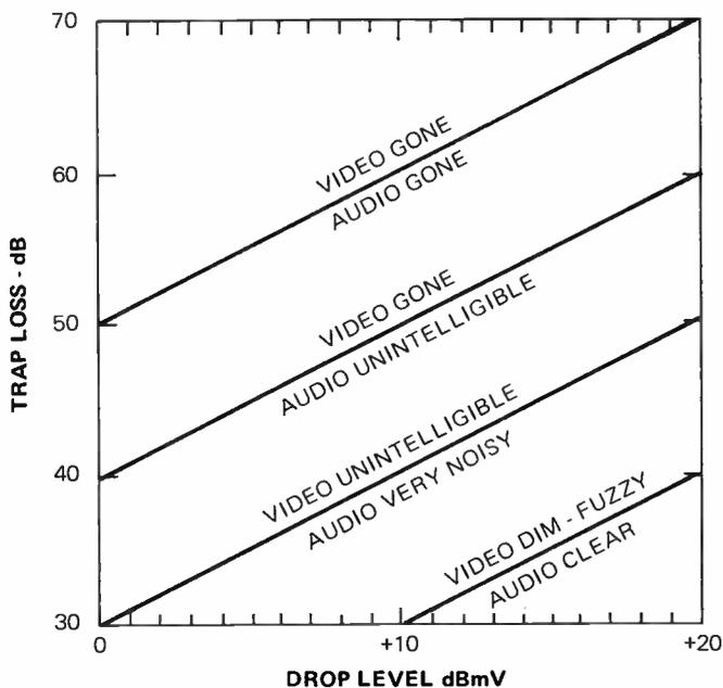
The best approach is to estimate the complaint percentage and plan this amount of very deep notch traps, or direct sound traps, in the mix of traps you'll buy.
