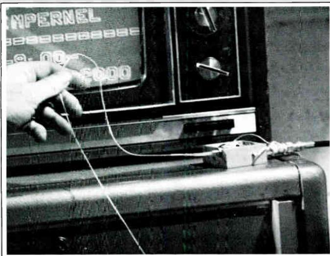
A single fiber sheathed in a plastic tube is shown connected to the Bell Northern receiver in the Teleprompter installation.
