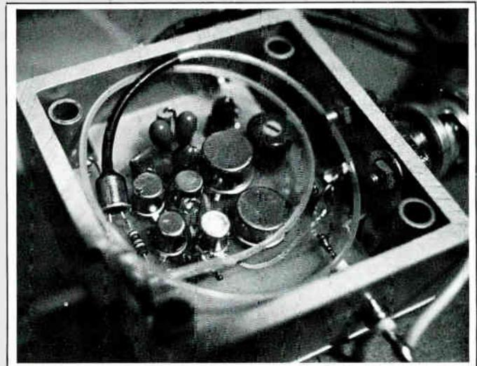
Inside the Bell Northern receiver, the P.I.N. diode can be seen connected to the end of the optical fiber with the video amplifier included in the same housing.
