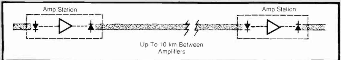
Typical Cable System Using Fiber Optics
