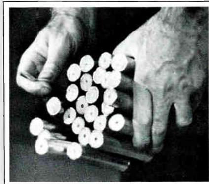
The six strand optical fiber cable can replace up to 20 conventional coax cables.
