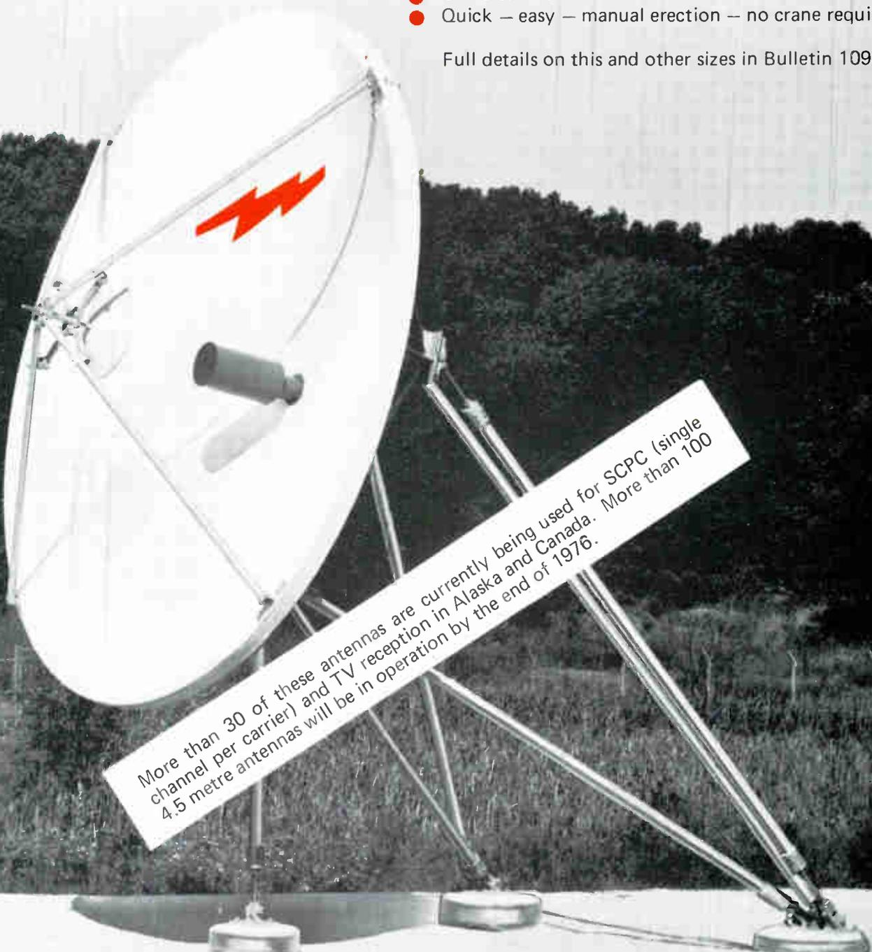
More than 30 of these antennas are currently being used for SCPC (single channel per carrier) and TV reception in Alaska and Canada. More than 100 4.5 metre antennas will be in operation by the end of 1976.
