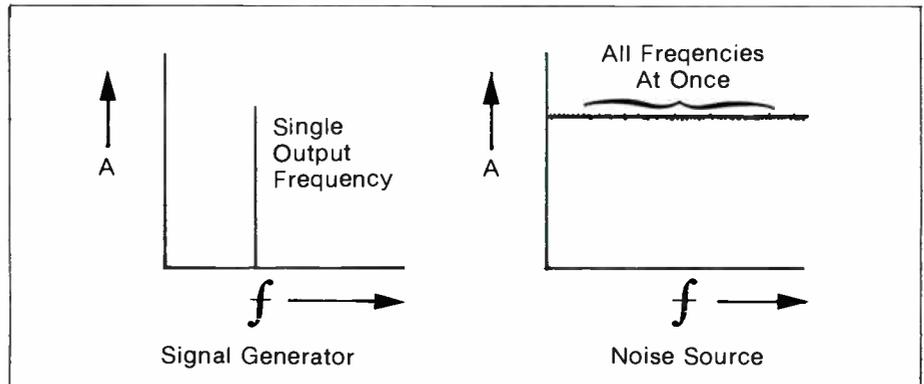
Figure 2—Difference Between Signal Generator and Noise Source.
