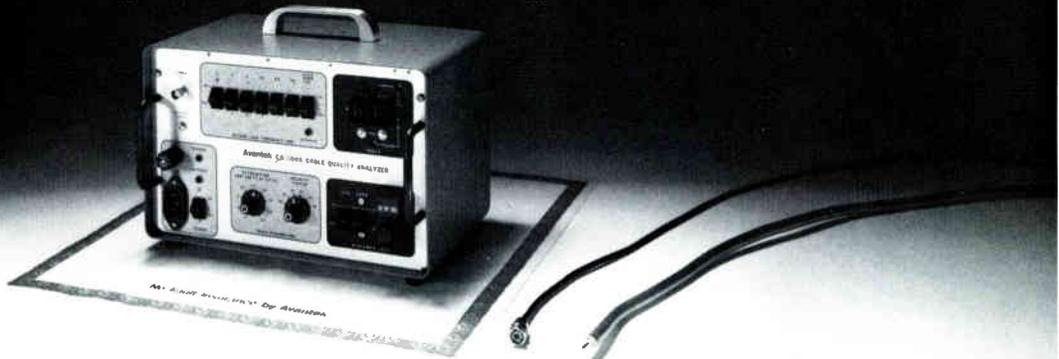
Now you can quickly and accurately isolate cable faults that might impair your CATV system's performance. Avantek's CA-100A Cable Fault Locator will identify those shorts, opens, crimps and parted center conductors as well as detect unauthorized drops.
