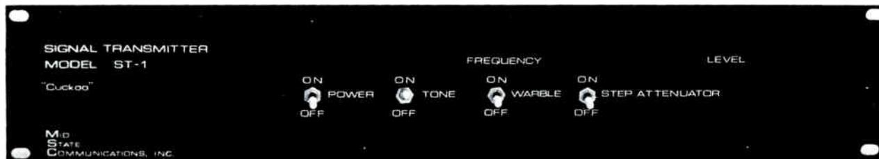
An ST-1 signal transmitter bolts into your headend, and produces an easily identifiable signal at any frequency from 86 to 110 MHz. The signal can be either FM modulated at 1 KHz or FM warbled, like a cuckoo clock. The cuckoo signal can be easily recognized even in a noisy environment. A standard FM radio is then used as a receiver. The sensitivity of the system depends on the quality of the radio you purchase.
