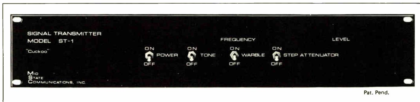
An ST-1 signal transmitter bolts into your headend and produces an easily identifiable signal at any frequency from 86 to 110 MHz. The signal can be either FM modulated at 1 kHz, or FM warbled, like a cuckoo clock. The cuckoo signal can be easily recognized even in a noisy environment. A standard FM radio is used as a receiver. The sensitivity of the system depends on the quality of the radio you purchase.
