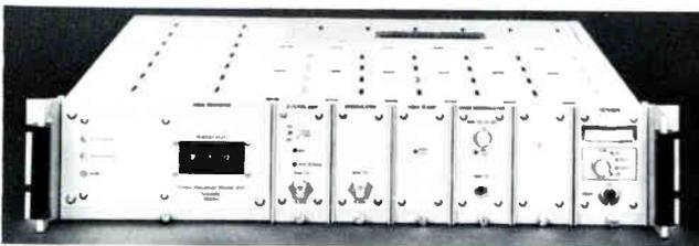
*New receiver designs such as this Scientific Atlanta model feature threshold extension.*
