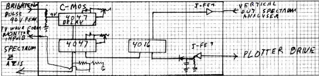
Schematic of sampling pulse generator.
