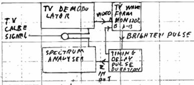
Block diagram of Field Setup.
