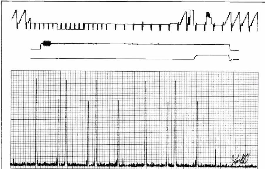
**Spurious Response**—Sampling each channel in the vertical interval produces a display without frequency components other than the picture and sound carriers. 30 kHz I.F. bandwidth was used. Vertical resolution is 20 dB per major block.
