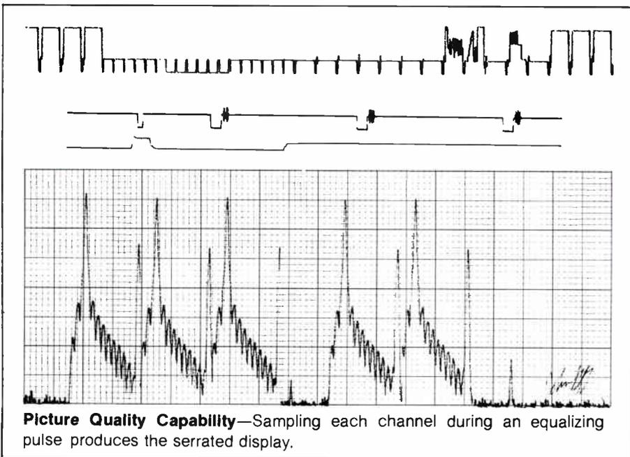
**Picture Quality Capability**—Sampling each channel during an equalizing pulse produces the serrated display.
