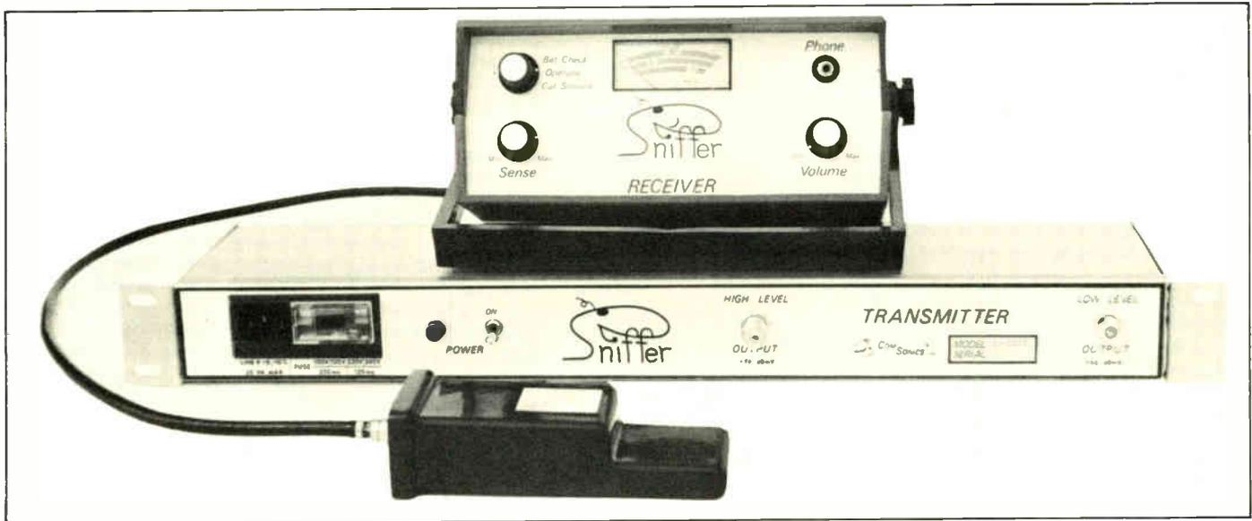
pinpointing and cleaning up shielding flaws is the purpose of a leakage detection system. Rapid leak location can be obtained only by equipment designed for near and far field detection, AND near field isolation.
