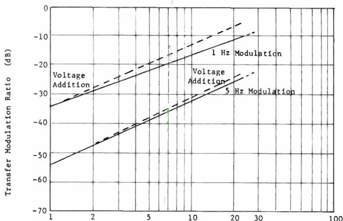
It can be seen that, if the amplifier non-linear distortion is insignificant, the length of an AGC/ASC amplifier cascade may be limited by the amount of transfer modulation that can be tolerated. The use of video carriers as the reference signals aggravates this problem, unless steps are taken, because of the presence of 60 Hz pulses in the video signal.
