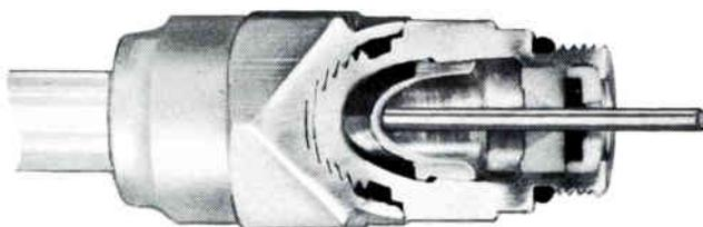
Now available from LRC a sealed feed thru aluminum connector. This new design eliminates the need for an expensive, more complex pin style connector. This connector provides a positive seal around the cable center conductor. A 40 psi moisture barrier is obtained from housing to cable for all three size cables.
