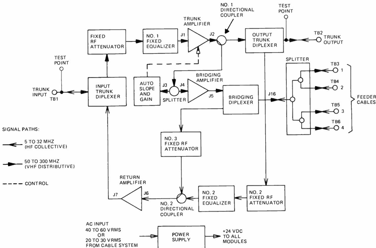
**Figure 3. Mark IV Station Block Schematic**
