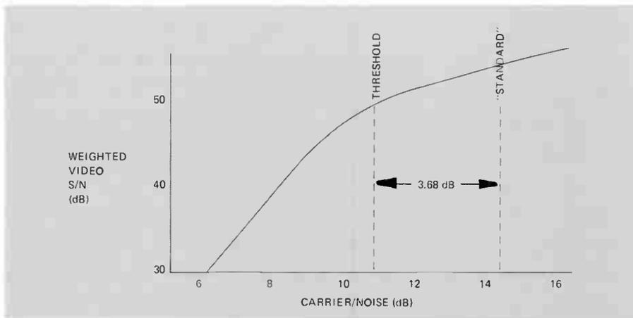
Figure 2 Typical Signal to Noise Performance as a Function of C/N
