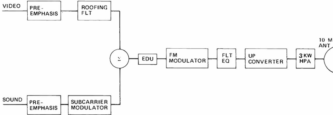
Figure 6 Elements of a TV Uplink Station
