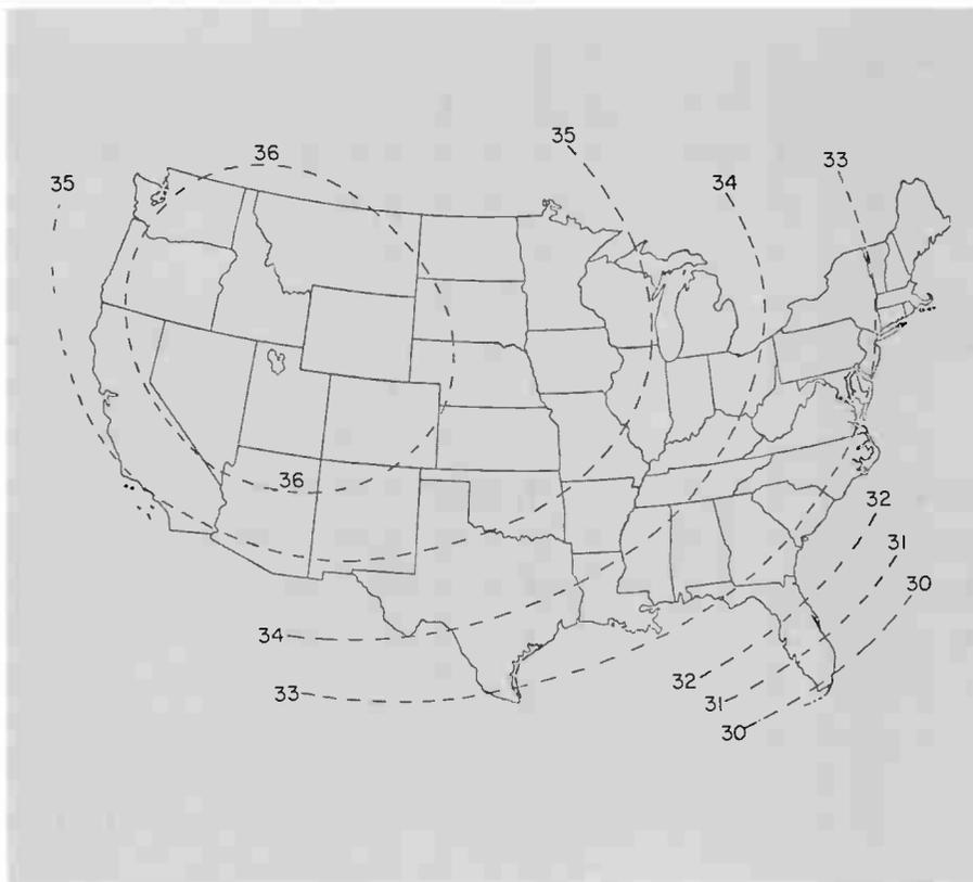
Figure 3 Typical Satellite Footprint Showing EIRP in dBW
