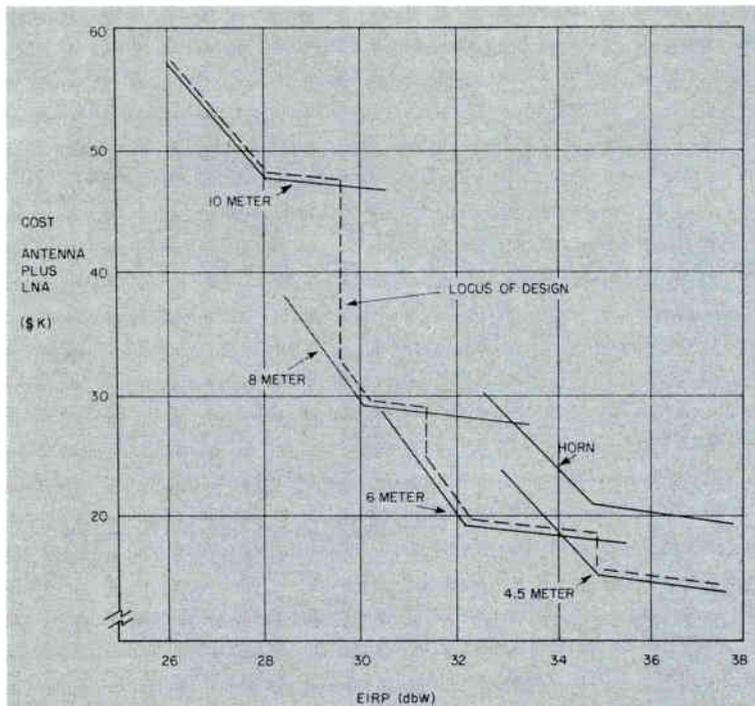
**Figure 6 Cost as a Function of Available EIRP Based on C/N = 14.68 dB Minimum**
