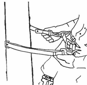
Figure 3: Position of the safety strap when in use
