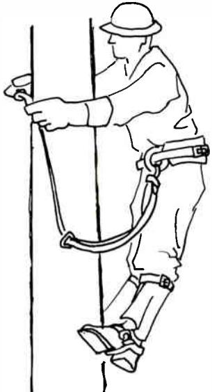
Figure 10: Passing the safety strap to the right hand
