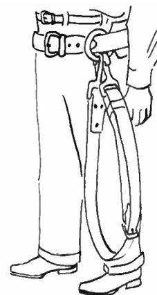
Figure 2: Position of the safety strap when not in use
