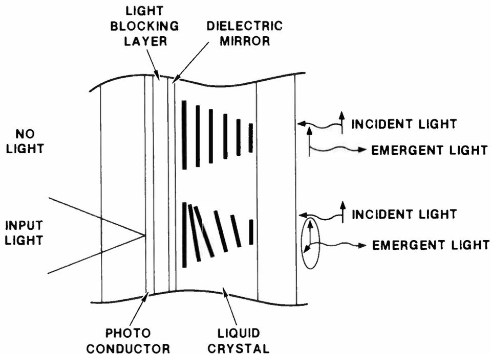
Figure 1: Functional diagram of the hybrid field effect liquid crystal light valve.
