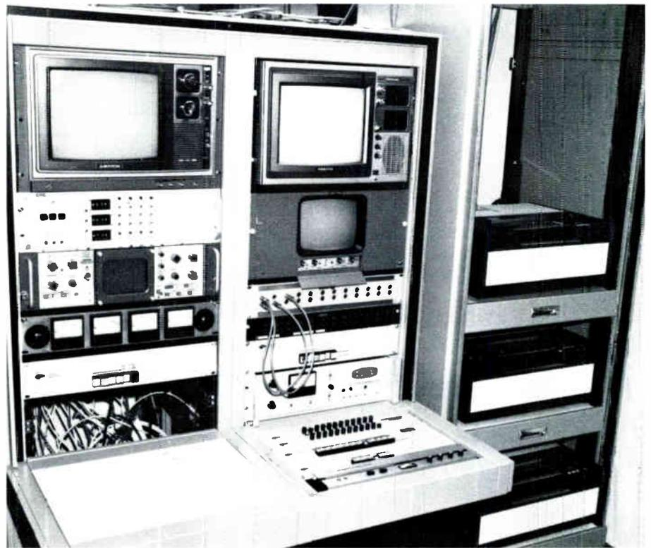
*This compact automated pay-cable installation uses commercially available 24-inch racks for videocassette machines.*
