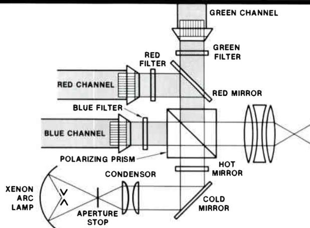
Figure 2: Schematic of liquid crystal light valve color TV projector.
