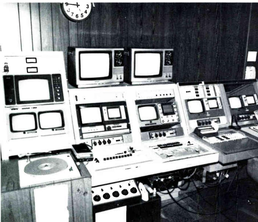
*This four-channel airing console includes local origination, automated sports and two automated pay channels.*
