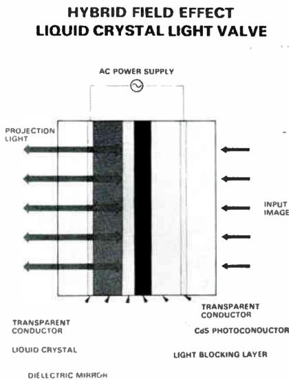
*Pictured above is a diagram of the hybrid field effect on the liquid crystal light valve.*
