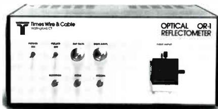
This new device is compact and portable (17" x 7" x 13"). Narrow pulse width allows one meter resolution. High gain PMT offers superior signal-to-noise ratio. The OR-1 accepts a range of fiber diameters up to 150 micrometers, and features an adjustable signal level and repetition rate.
