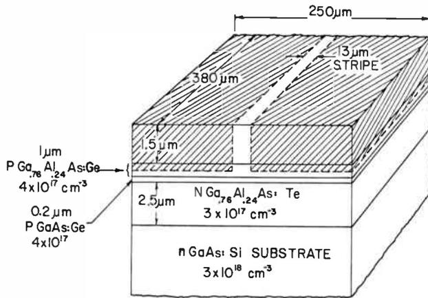
Figure 1. Layer Structure of the Stripe-Geometry Double Heterostructure Laser.
