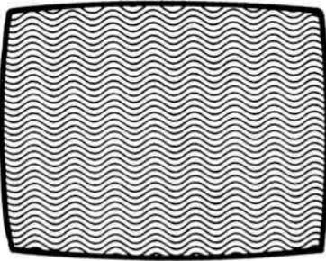
**Q** I have a Channel Commander 1 headend and have had problems with beats in the picture. The beat appears on channel 8 when channel 9 is on and disappears when I turn channel 9 off. I have seen this kind of problem at other headends that I've worked on and have usually been able to cure it by one means or another. This one is stubborn though. Thanks for any help you can give.
