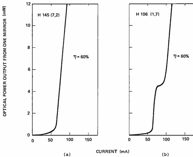
Fig. 2 Output Characteristics of Linear and "Kinked" Lasers.
