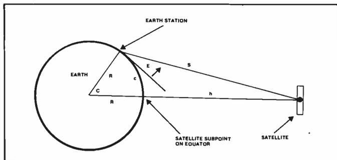
Cross-section representation of the earth showing the earth station/satellite relationship. The angle of great-circle arc, **c**, is the same as that shown before, and is equal in degrees to included angle **C**.
