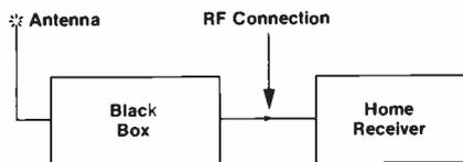
Figure 4: functional block diagram of home receiver with external black box for caption insertion.
