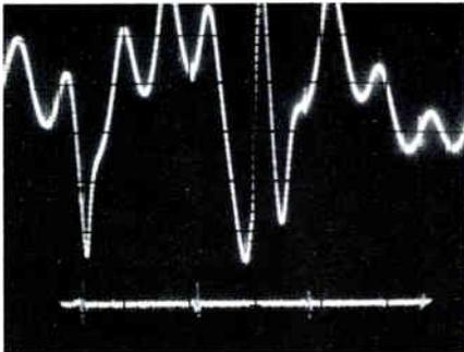
Figure 6: magnified sweep response—with "TEST" type trap. Note narrowed sweep width.
