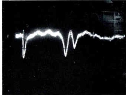
Figure 6A: magnified analyzer response—with trap - narrow sweep width.
