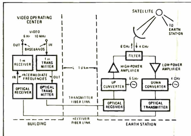
Figure 1. Transmitter/receiver system in Bell's test can interchange the fiberoptics links (shown) with coaxial cable for comparing transmission and reception characteristics.
