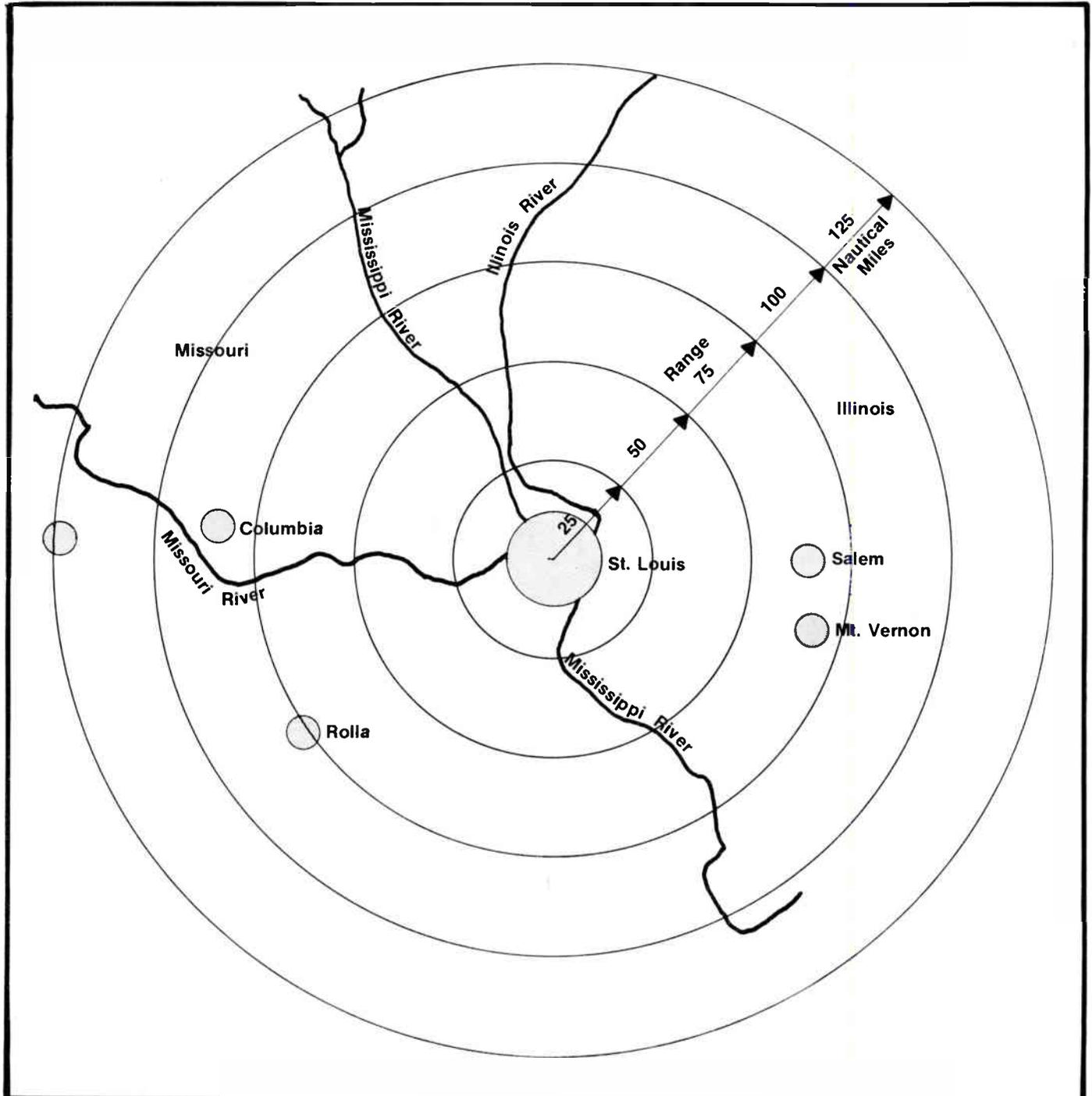
The Radar echo around St. Louis is "ground clutter" caused by local radar reflection from buildings. Other echoes are precipitation.
