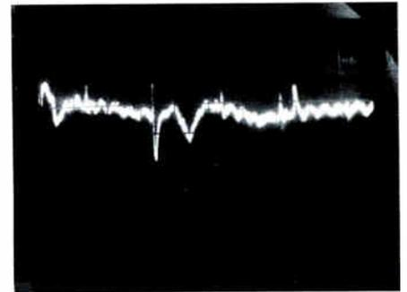
Figure 2A: analyzer response—TV set on channel 3. Note additional response at 50 MHz, and TV local oscillator.
