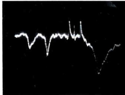
Figure 7A: analyzer response—TV channel 4 and antenna resonant at 160 MHz.
