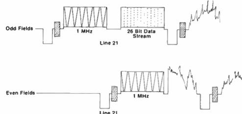
Figure 1: NBS proposed signal format.
