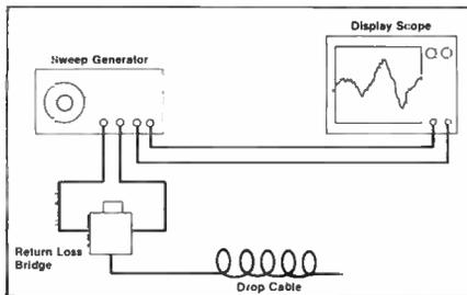
Figure 8: equipment setup for swept return loss measurement.
