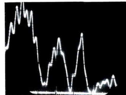
Figure 4: sweep response—converter brand X. Note multiple response pattern.
