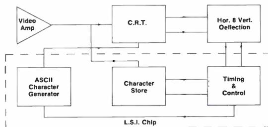
Figure 3: functional block diagram of home receiver modified to provide captioning for the hearing impaired.
