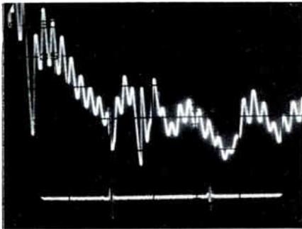
Figure 5: sweep response—channel 4 with "TEST" type trap.
