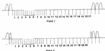
Figure 2: 525-line television waveform showing field blanking interval.
