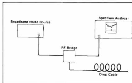
Figure 9: alternate setup using noise sound and spectrum analyzer.
