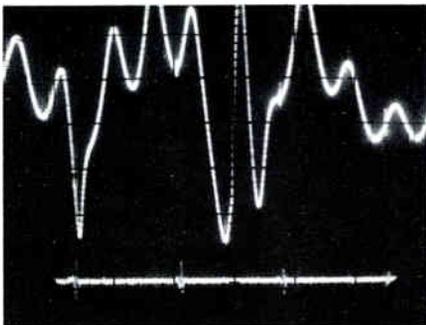
Figure 6: magnified sweep response—with "TEST" type trap. Note narrowed sweep width.
