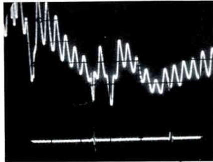
Figure 2: sweep response—TV set on channel 3. Note additional response at 50 MHz, a quirk of the tuner.
