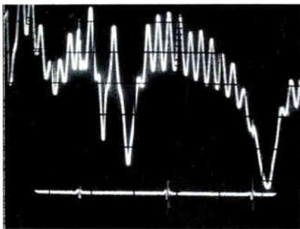
Figure 7: sweep response—TV on channel 4 antenna connected to transformer resonant at 160 MHz.
