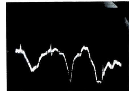
Figure 4A: analyzer response—converter brand X. Note multiple response pattern.
