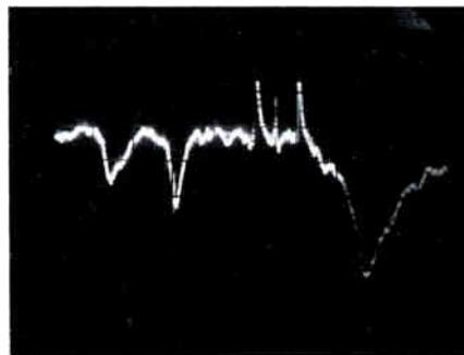
Figure 7A: analyzer response—TV channel 4 and antenna resonant at 160 MHz.
