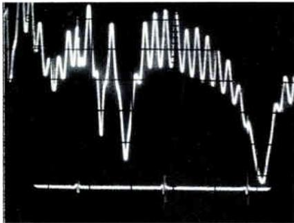
Figure 7: sweep response—TV on channel 4 antenna connected to transformer resonant at 160 MHz.
