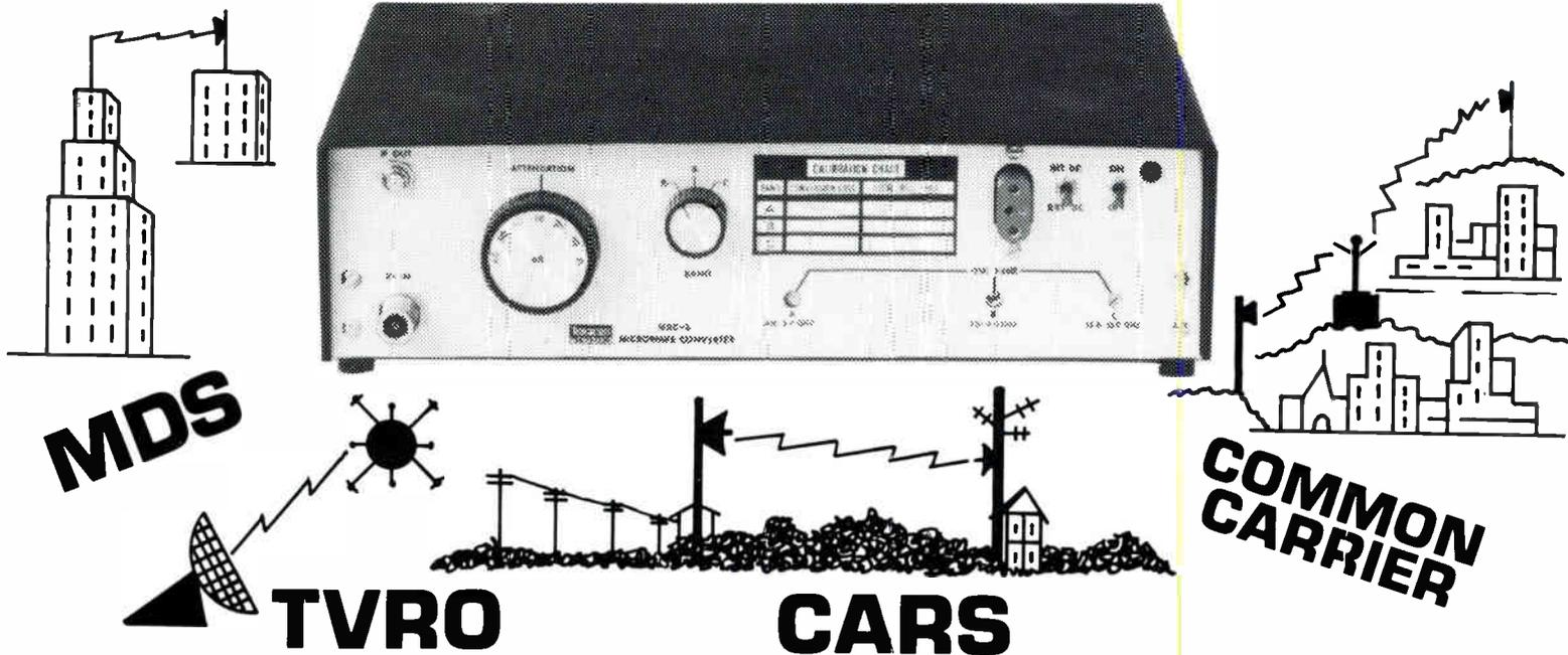
Texscan's microwave down converter permits measurement in the MDS (2.1 GHz) TVRO (3.7 GHz) and CARS (12.7 GHz) band with existing VHF test equipment. Spectrum analysis, signal strength and even microwave sweeping are possible with the MDC-3.
