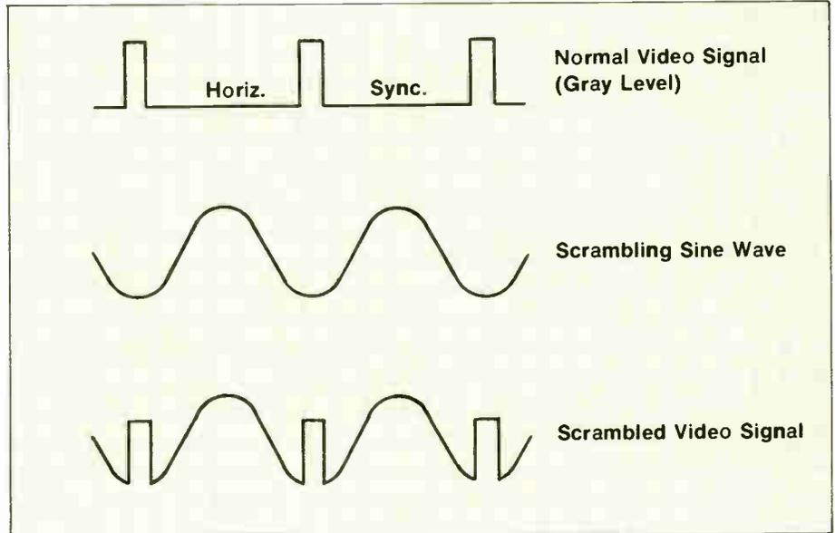
Figure 1.2: Scrambling waveforms
