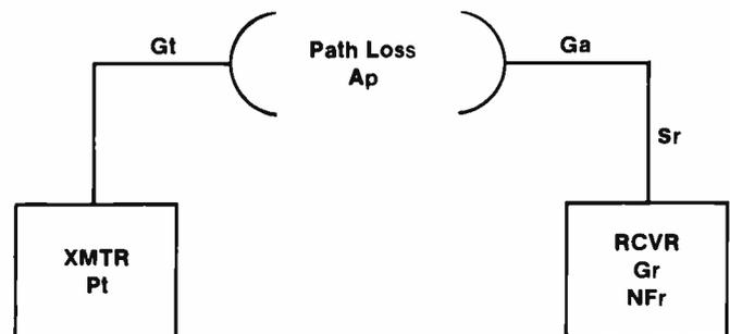
Figure 1: MDS system diagram
