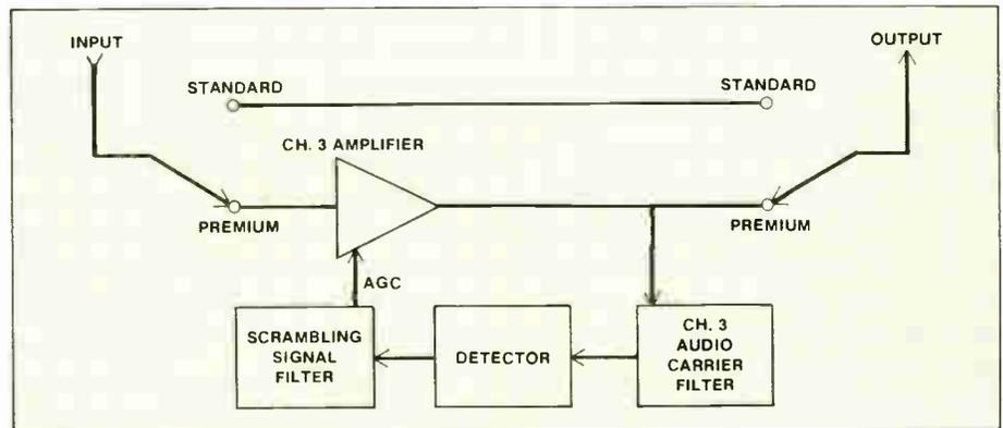
Figure 1.3: Mini-code block diagram (premium Channel 3)
