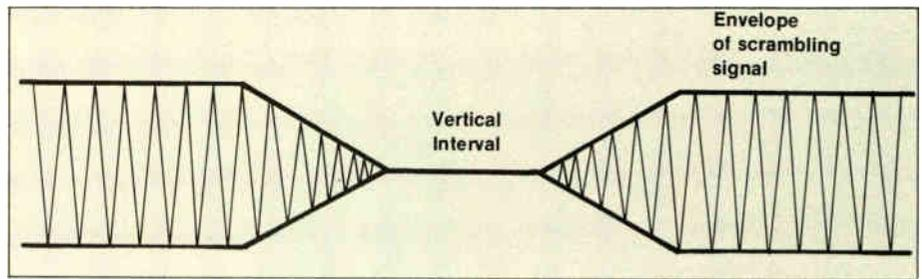
Figure 2.3: Vertical interval suppression of scrambling
