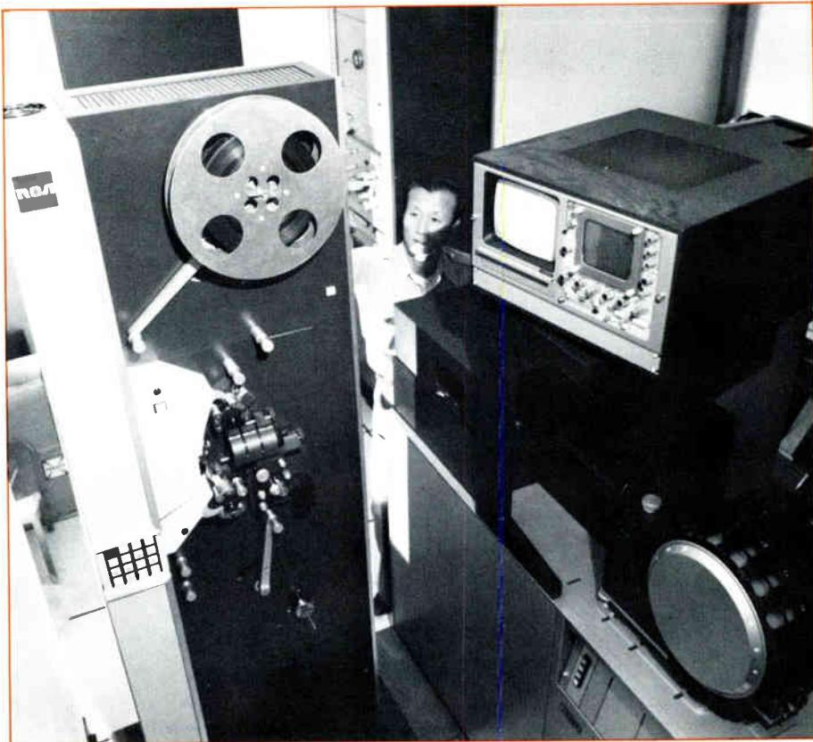
The film island (at left) is the RCA FP-35B 35mm film projector. At right is the dual drum RCA TP-7 35mm slide projector. In the background is the RCA dual 16/35mm sound dubber.
