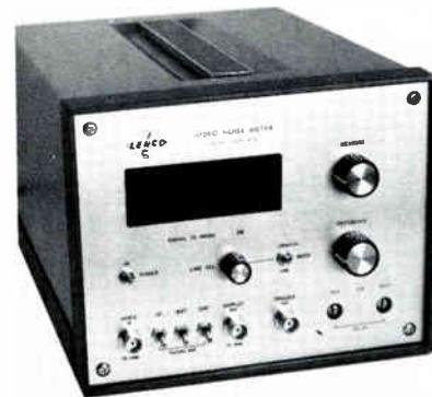
A major feature of the VNM-428 is its ability to make accurate, real-time signal-to-noise measurements of any composite video signal no matter what the source. The noise meter has a built-in calibrator that ensures accuracy of ±0.5 dB throughout the range of 20 dB to 55 dB. The signal-to-noise ratio is calibrated to EIA standards and is shown on a large LED display.
