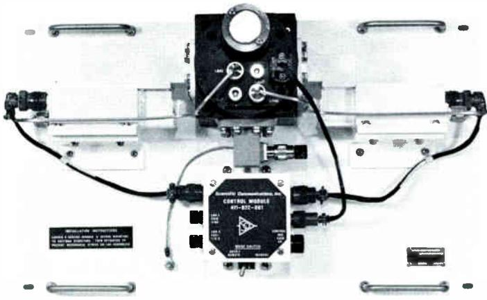
The SCI Model SCF-306 Series Redundant GaAs FET Low Noise Amplifier Assembly provides amplification of RF signals in the 3.7 to 4.2 GHz frequency range. The assembly consists of two GaAs FET amplifiers, a low loss transfer switch, and a transfer switch control module. The entire system is mounted on a single plate designed for mounting near the antenna. Interface connector pins provide system status information for remote monitoring.
