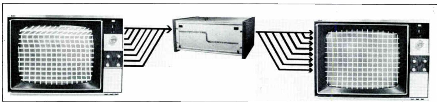
Typical hooking distortion (left) and after time base correction (right).
