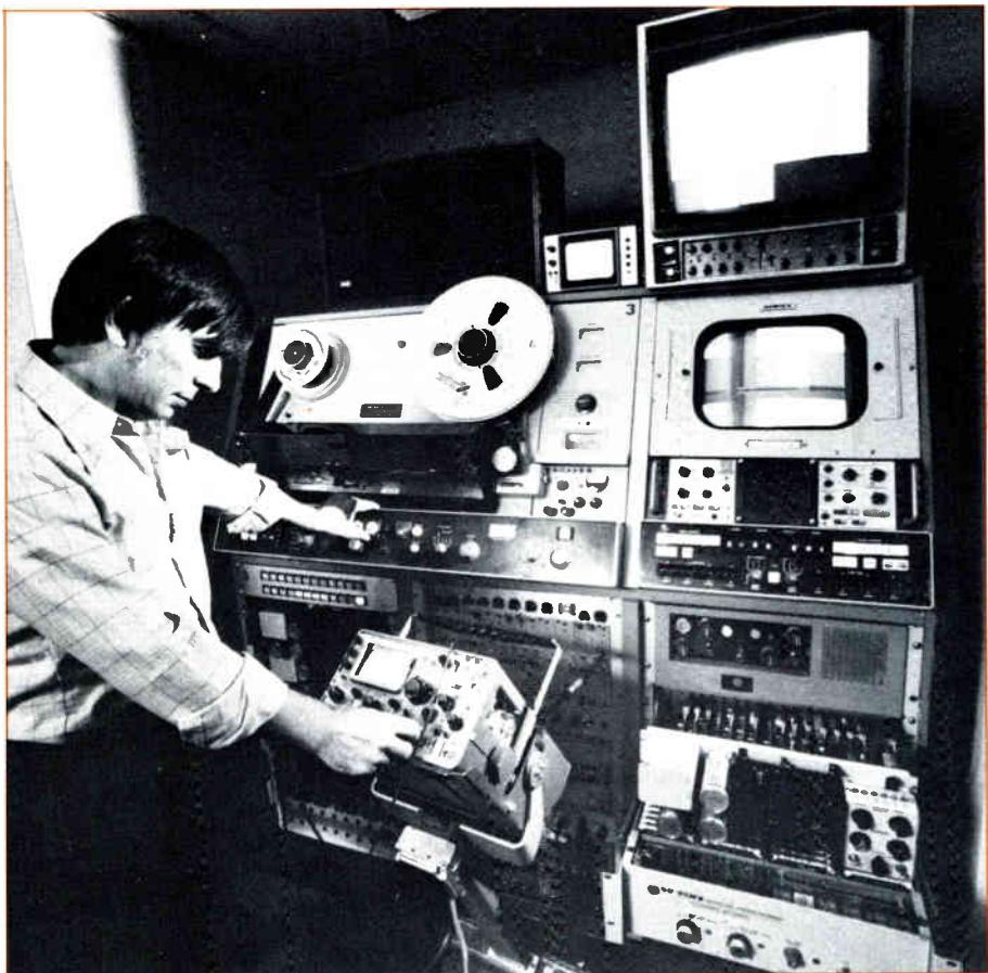
One of 14 two-inch quad videotape recorders used for edit and on-air transmission.
