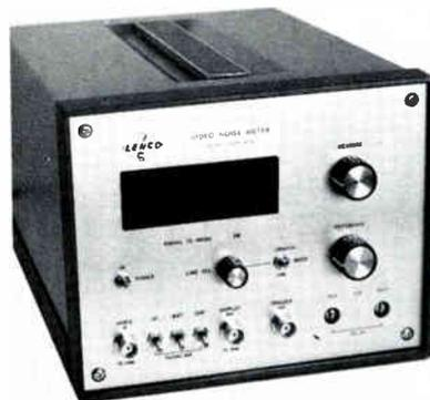
A major feature of the VNM-428 is its ability to make accurate, real-time signal-to-noise measurements of any composite video signal no matter what the source. The noise meter has a built-in calibrator that ensures accuracy of  $\pm 0.5$  dB throughout the range of 20 dB to 55 dB. The signal-to-noise ratio is calibrated to EIA standards and is shown on a large LED display.
