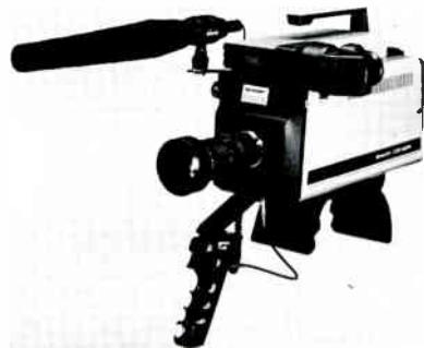
A key feature of the new camera—model XC-320U—is a rugged, unified moulded housing block which contains the lens, beam splitter, coil assemblies and tubes. The three vidicon tubes are attached directly to the dichroic mirror. As a result of the rugged design of the block, registration problems have been completely eliminated.
