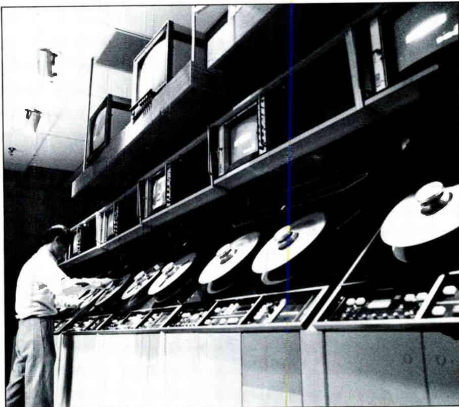
RCA Americom's bank of seven two-inch quad VTRs, used for playback and post-production programming.
