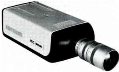
handling capability and yield clean, clear images of moderate contrast even with backlighting or light flare. Auto-sensitivity control extends the dynamic illumination range to 10,000:1. Auto beam current control compensates for normal aging of the pickup tube.
