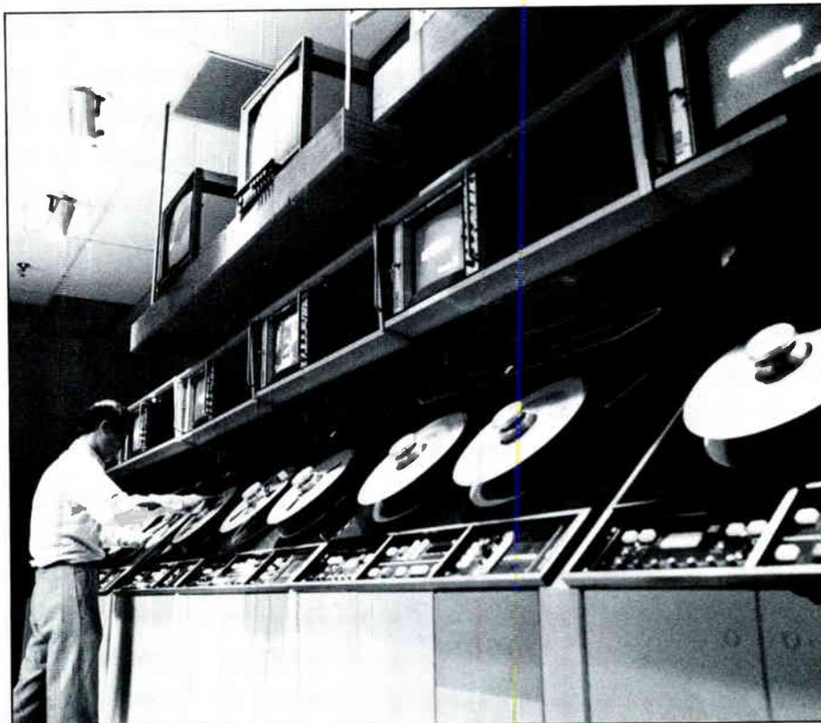
RCA Americom's bank of seven two-inch quad VTRs, used for playback and post-production programming.
