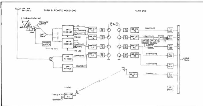
Figure 1: A typical 1978 CATV network.
