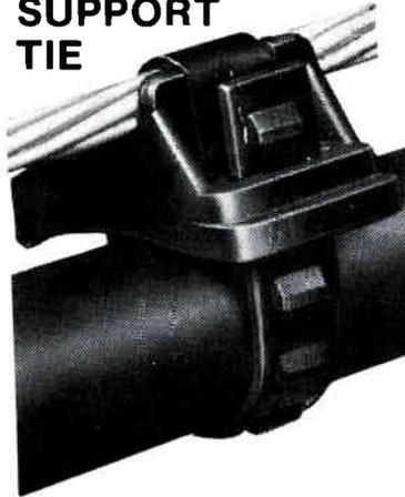
Attaches CATV Coaxial or Telephone Cable to the support strand to form the expansion loop and keep equipment and cables clear of pole hardware.
