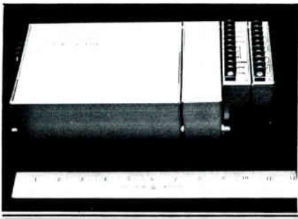
*The Universal Addressable Data Terminal (UADT) is shown with a cable and premium module, security module and energy control module. RF and power are applied on the left hand connectors.*
