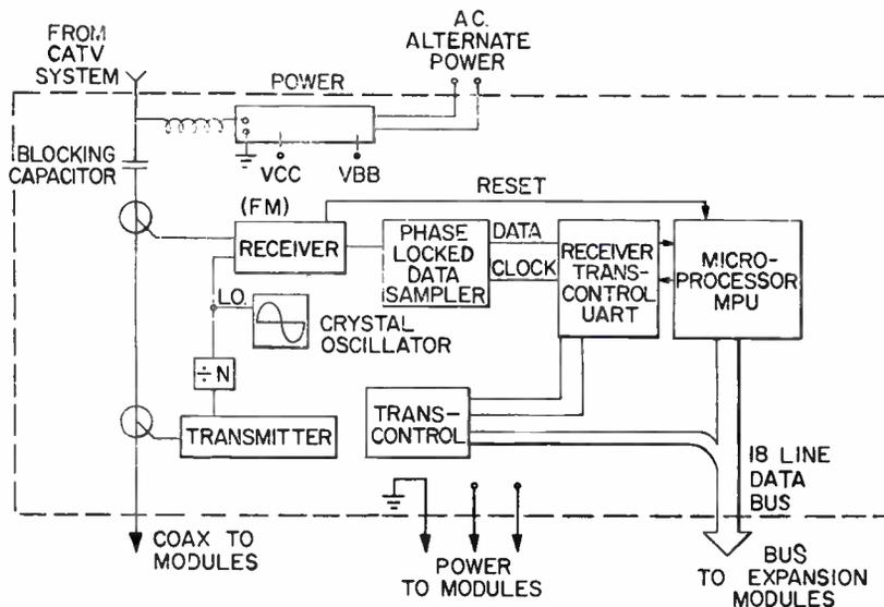
*Block diagram of the home terminal (UADT). Shown is the interlaced receiver transmitter.*
