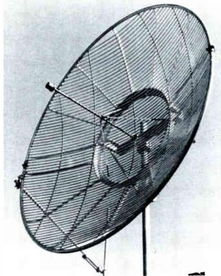
In addition to installation and alignment ease, antenna efficiency is a minimum of 55 percent; cross polarization discrimination is typically at 35 to 40 dB at 0 degrees azimuth and windload characteristics are 25 percent (below 1000 MHz) and 40 percent (above 1000 MHz) of an equivalent solid parabola.
