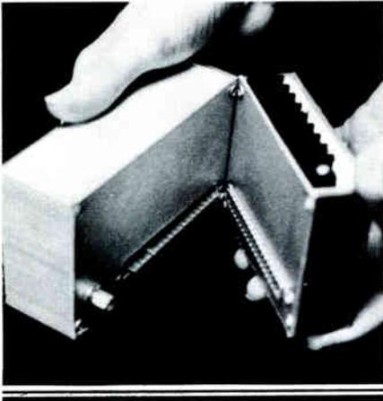
*The bus is carried through all modules. The modules can be connected Daisy Chain fashion, and up to 256 modules can be stacked onto one UADT.*
