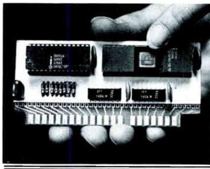
*A single chip computer and a programmable P/SART are the brain for the home terminal. Address recognition, control and self tests are supervised by this module.*
