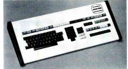
communication. Tentative edits are entered into a decision list for preview, modification or recording. Any list entry is instantly accessible for review or modification. Insertions or deletions may be made at any time with completely automatic recomputation of all record times and the total duration. System status, together with the complete decision list, is viewable at the operator's console monitor.
