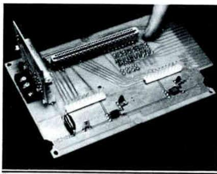
*The motherboard has positions for the MPU, receiver, transmitter and the power supply. RF stripline carries cable through to the home with taps for the receiver and transmitter.*
