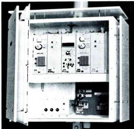
The DM18 Digital Radio is offered as a complete microwave communications system. Transmitters, receivers, enclosure, alarm system, antennas, multiplexers and installation are all available from Farinon.
