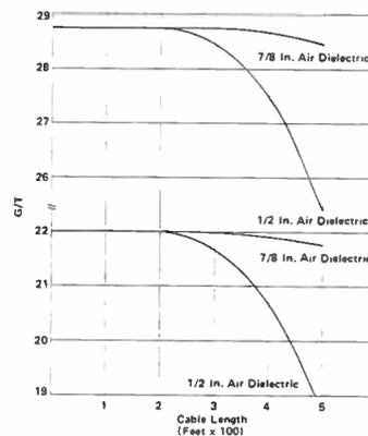
Figure 1: System G/T versus post LNA cable length.
