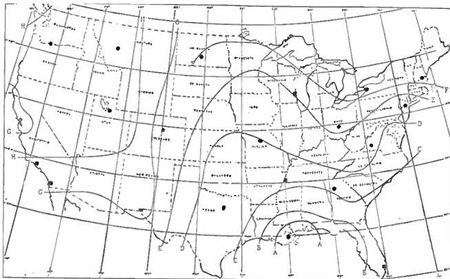
**Figure 4: Contours of equal precipitation attenuation.**
