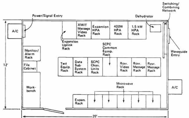
Figure 6: Typical shelter equipment layout.
