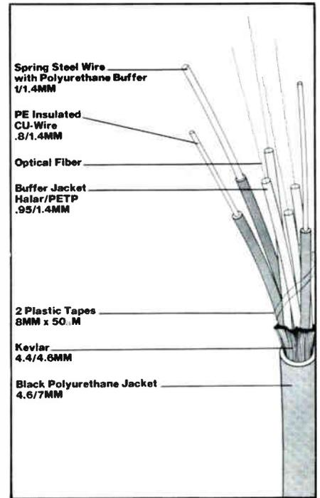
A cross-sectional drawing of Siecor's fiberoptic cable.
