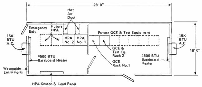
Figure 4: Electronics equipment shelter floor plan.
