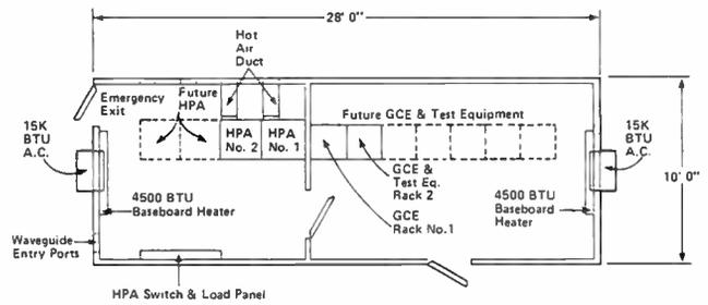
Figure 4: Electronics equipment shelter floor plan.
