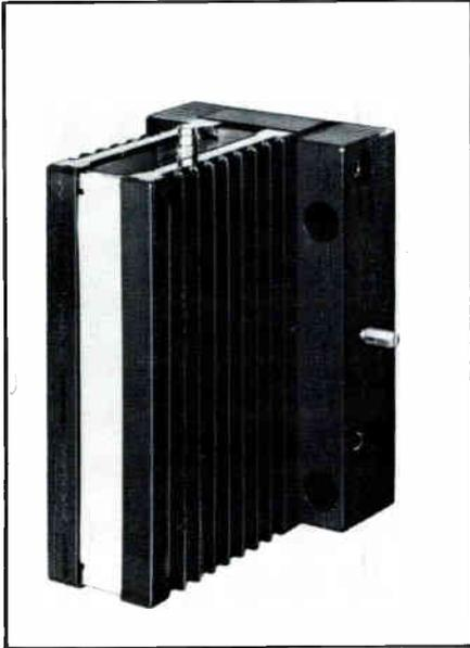
The fiberoptic transmitter (above) and the transmitter with power supply (below) are used in the Joplin cable television fiberoptic trunk system. The receiver units are identical in size and appearance.
