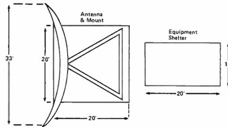
Figure 5: Typical message/video T/R earth station layout.
