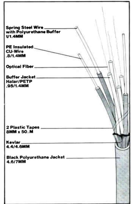
A cross-sectional drawing of Siecor's fiberoptic cable.
