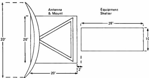
Figure 3: Typical redundant T/R earth station layout.
