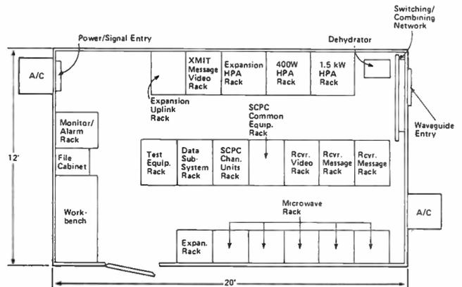
Figure 6: Typical shelter equipment layout.
