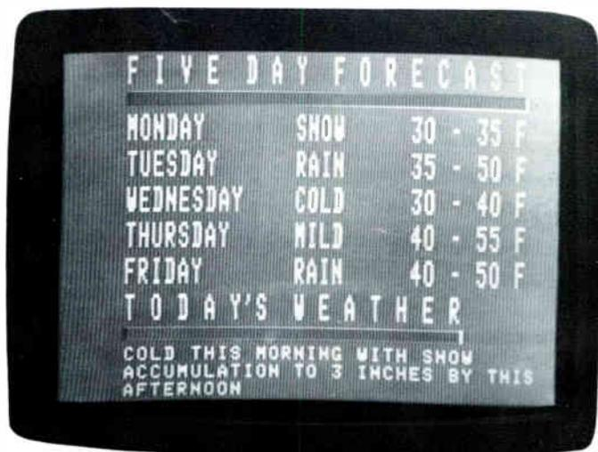
*Typical Info-Text "electronic newspaper page" is weather report, which is selected and displayed by homeowner by pressing button on special decoder attached to his TV receiver's antenna terminal.*
