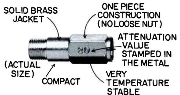
LRC Attenuator Pads are available in values of 3, 6, 10 and 20 db with an accuracy of 5% or  $\pm .5$  db.
