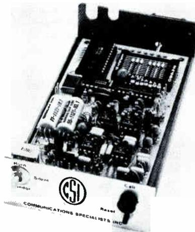
Well protected circuitry and matrix switch code settings are provided for ease of installation. Relay outputs give isolation and eliminate extra parts required for installation.
