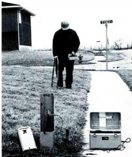
An engineer uses the A-shaped earth contact frame with the Dynatel 573 to find underground cable sheath faults. By simply checking the meter built into the hand-held receiver, the G.E. Cablevision engineer can tell if the fault lies ahead or to the rear on the cable run.
