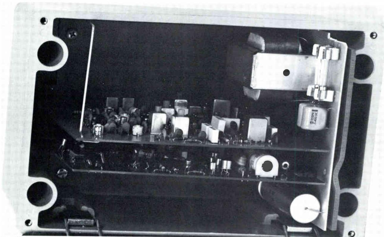
*Scientific-Atlanta's radio receiver/carrier current transmitter receives the message from the message generator unit via a standard cable drop.*
