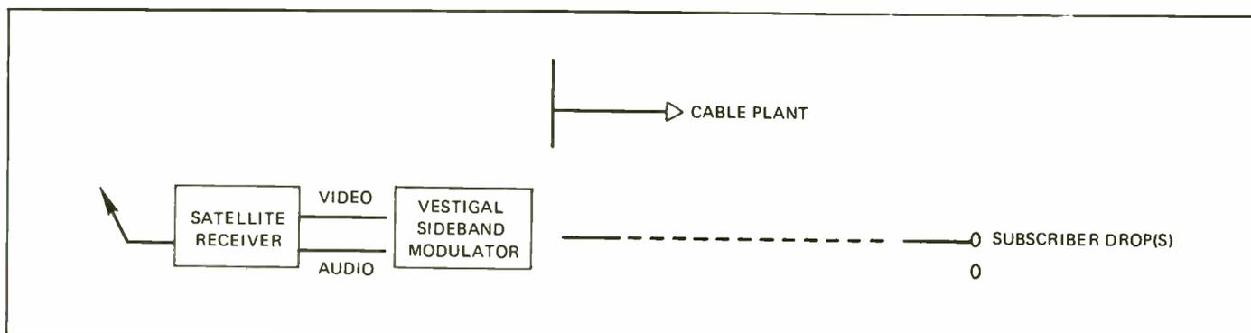
Figure 1: Satellite feed to CATV system.
