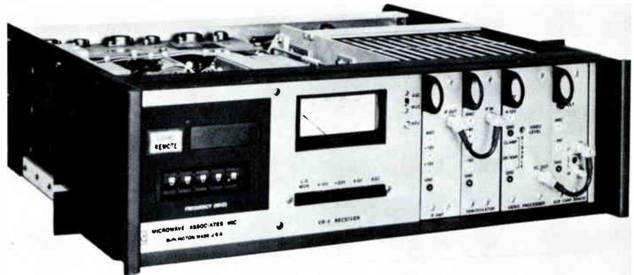
with its quarter megahertz frequency stepping synthesizer. The receiver is the same general size and appearance as Microwave's VR-3. It also uses the same plug-in modules resulting in a compatibility of appearance and operation. The VR-4 is compatible with the PAC-5 or PAC-6 series subcarrier demodulators, enabling the operator to receive additional voice, slow scan video or data subcarrier material.
