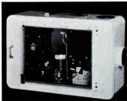
One of the company's newest products was the 60594 earth station video receive equipment—a compact, solid state weather protected downconverter. This downconverter is designed for direct mounting on earth station antenna to convert incoming satellite signals in the 11.7 — 12.2 GHz range to a 70 MHz IF output. The 70 MHz output connects to the optional baseband treatment equipment with up to 500 feet of low cost coaxial cable, without
