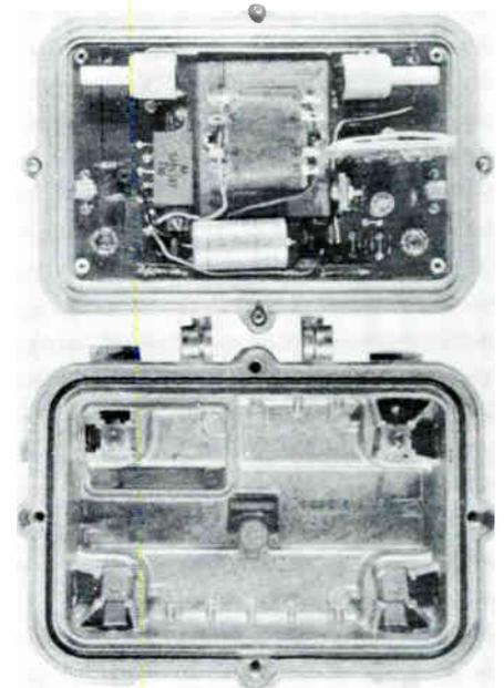
The company also showed its recently introduced MX-5-ULE utility line extender. This device is designed for applications where a low-price line extender is desirable. The one-way line extender features low initial cost and low power consumption. The MX-5-ULE utilizes a high efficiency power
