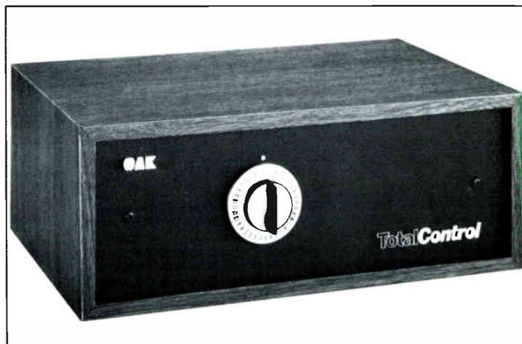
Oak's "TotalControl" converter/decoder is a unique 35-channel device, designed for one or more pay-TV channels, up to 35 channels. With this new addressable unit, an operator can remotely control premium programming for each subscriber at the control center, ensuring total system security. The unit features automatic frequency control and a single detented rotary selector to control both basic cable channel selection and automatic pay channel descrambling.
