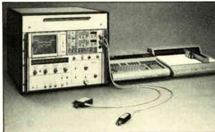
The 5610 makes measurements without interruption. Because the sweeper, SWR Autotester, Detector and programming all cover the 10 MHz to 18 GHz range, it is unnecessary to
