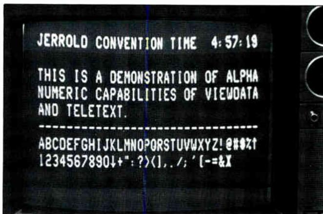
*Simulation of the alpha-numeric graphic capability of a Teletext 1 viewdata system.*
