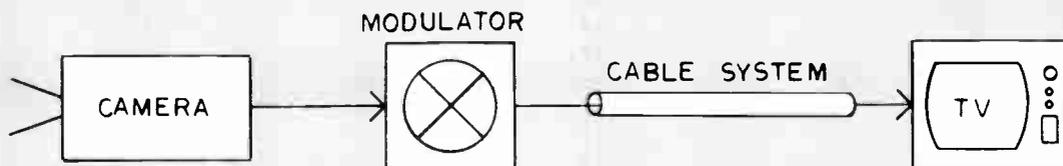
Figure 1. Traditional system for distributing television pictures.
