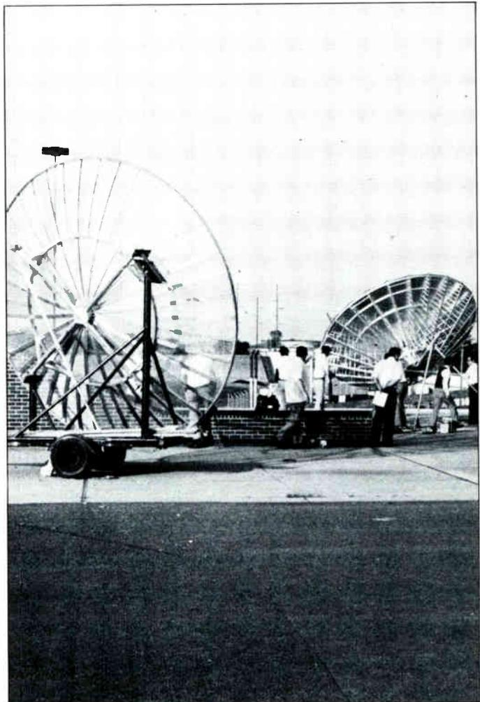
Six separate 10- to 13-foot antennas were operational during SPTS '79, most priced in the \$1,500 to \$2,500 range. Every reflector surface from screening to fiberglass and metal was evident.
