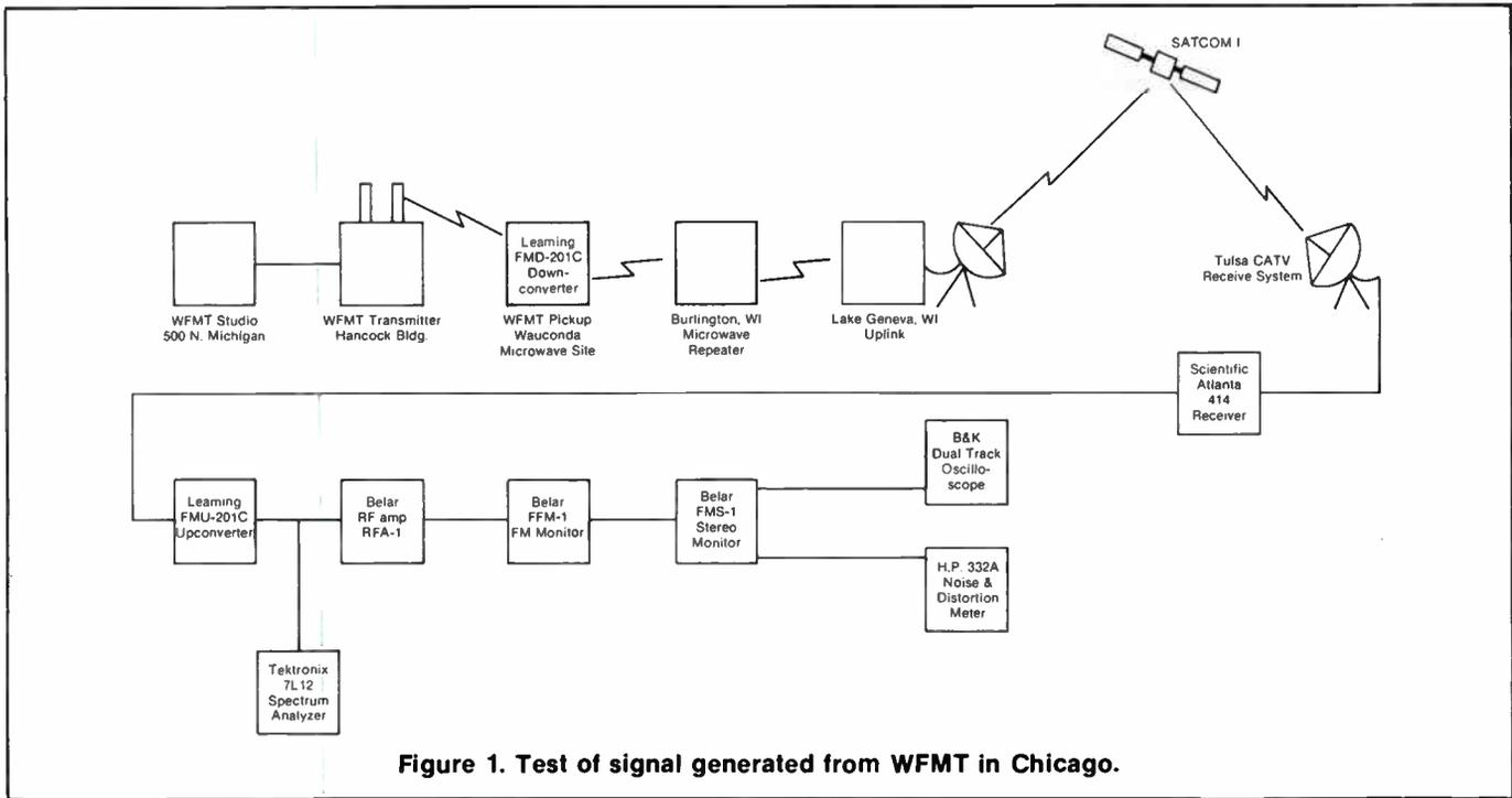
Figure 1. Test of signal generated from WFMT in Chicago.
