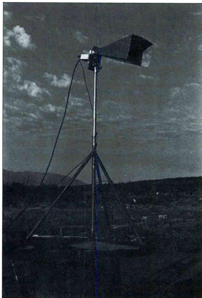
*The Feed for Spherical antenna developed by Swan is approximately 23 inches long. By placing multiple feeds in front of the antenna, simultaneous reception from several satellites is possible.*
