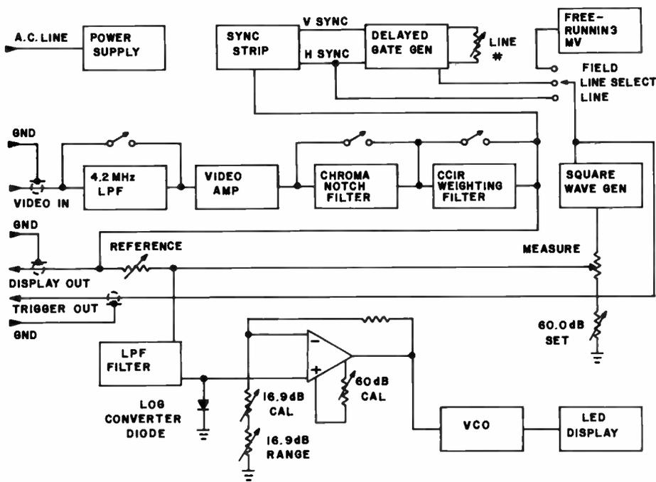
Figure 3. VNM-428 video noise meter functional block diagram.
