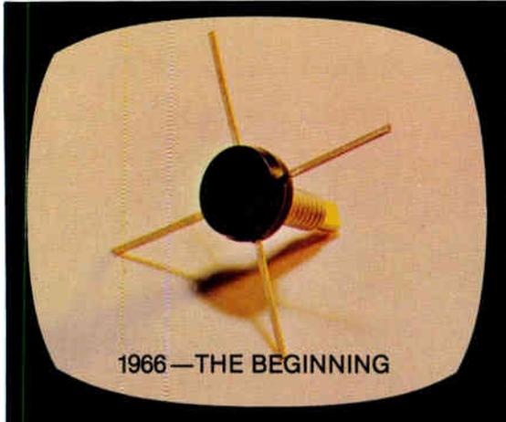
First transistors made and characterized especially for CATV amplifiers.
