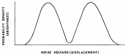
Figure 2a. Noise traces separated by more than twice their RMS levels.
