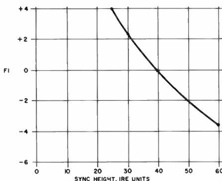
**Figure 5. Factor F1 versus sync height.**
