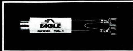
**The Eagle Matching Transformer TM-1** features in its rugged unitized construction a twin lead crimped and soldered to lugs, three (3) capacitor isolation for 1000V surge protection and a band width of 50 — 300 MHz in VHF and 470 — 850 MHz in UHF. Superior balance characteristics also highlight Eagle's high-performance matching transformer.
