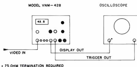
**Figure 6. Connection of VNM-428 for typical use.**
