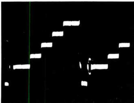
Figure 1c. Square wave amplitude just equal to twice rms noise.
