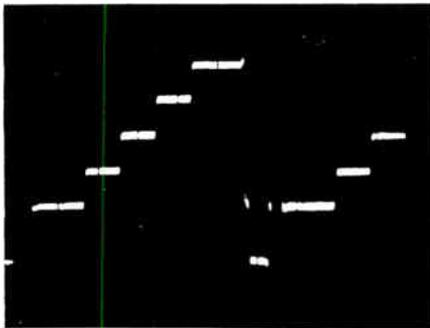
Figure 1a. Typical video waveform with SNR=approximately 39 dB.
