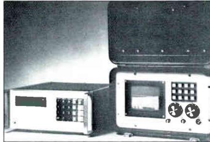
swept signal has been detected and the resultant waveform stored, the battery-saver circuit will shut down any circuits not required for the storage and display of the waveform; these circuits will remain deactivated until the microprocessor re-energizes them when it is time to receive and process the next signal. The battery-saver circuit increases the life of the rechargeable battery to about 3 hours between
