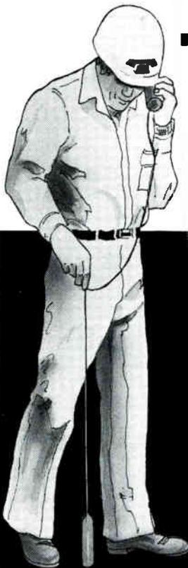
Underground television cables—energized or de-energized—are easy to trace with the Model 210 Line Finder™ from Radar Engineers. A clearly audible signal cuts out when the search wand is over the cable. It's just as simple to determine cable depth. Complete instructions are included—no special training or experience necessary.
