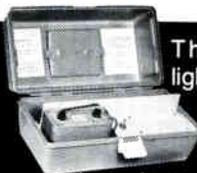
The Line Finder™ is rugged, lightweight, portable—everything a service crew needs to trace buried cables in one compact package. It goes anywhere, sets up in seconds, and needs no complicated adjustments. New circuitry virtually eliminates 60Hz interference. Call or write for more information and prices.
