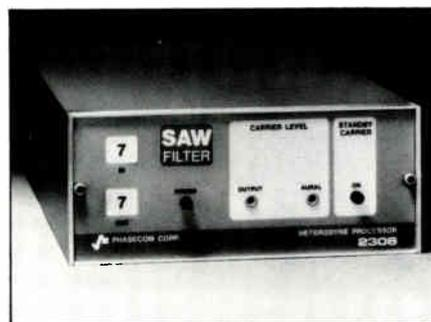
This model also incorporates Phasecom's "Automatic Notch Control" circuits which maintain the constant visual/aural carrier ratio, preset by front panel control. Only the amount of aural carrier attenuation needed to attain the desired carrier ratio is introduced at the IF passband, thus avoiding the conventional trap circuits that give rise to excessive group delay and color subcarrier attenuation.
