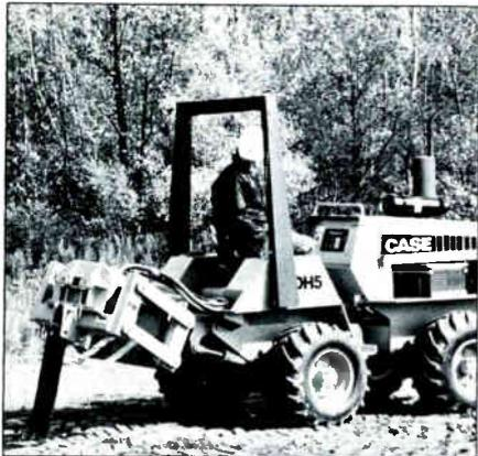
As on all Case line-layers, the line-layer itself attaches to the drive unit with an eight-point suspension system with rubber bushings to isolate the vibration from the drive unit and operator.
