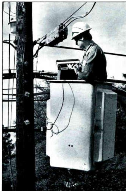
The radar-based device operates on either AC or DC with internal rechargeable batteries, and locates and indicates the distance to single or multiple faults or taps from one foot to 80,000 feet away. Variable pulse widths and continuously variable horizontal shift and horizontal magnification to 5X are said to provide clarity and precise viewing of the display, according to the Biddle Company.
