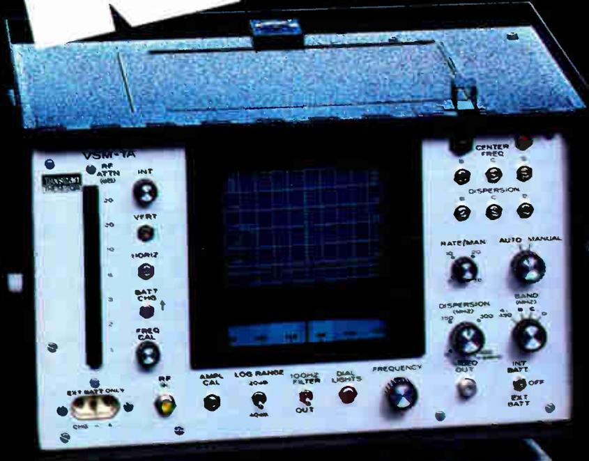
**TEXSCAN'S NEW VSM-1A VISUALLY DISPLAYS THE TOTAL FREQUENCY SPECTRUM FROM 4 to 450 MHz — PROVIDING FAST AND CONVENIENT ANALYSIS OF CATV SYSTEM PROBLEMS.**
