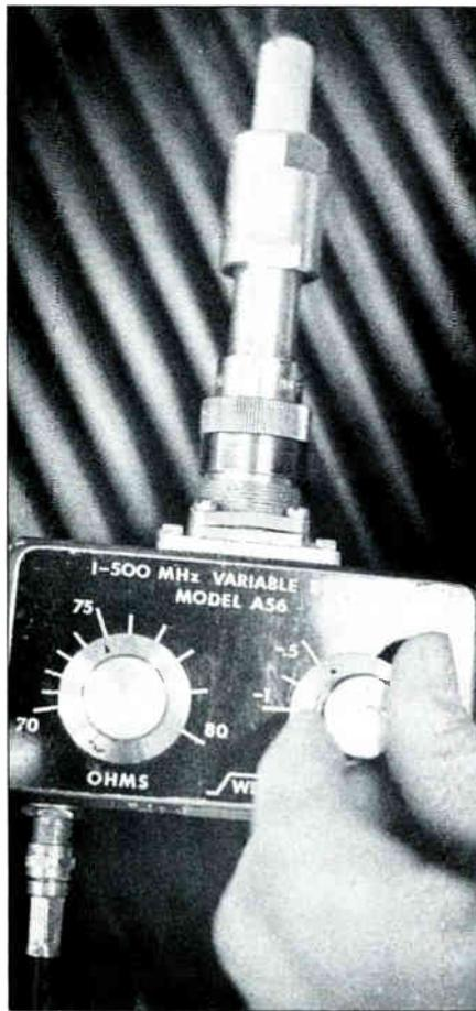
load measures 1.05 VSWR (32 dB) and the load VSWR is 1.26 (19 dB). This assumes a cable with no extraneous losses and  $Z_o = Z_s$ .
