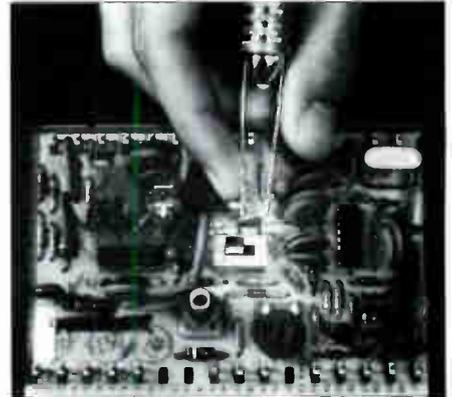
The Desco lighted tweezer is designed for working in poorly lighted field situations.
