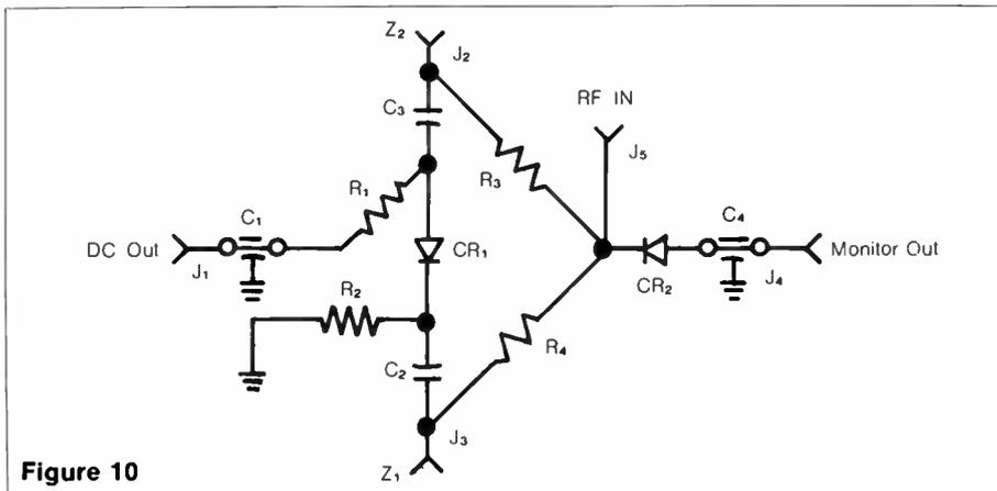
which is proportional to the value of  $R_x$ . In order to measure RF from A to B, a diode and RF decoupling return network is connected across A and B. A schematic of one make of return-loss bridge, Texscan's model RCB-3/75, showing all components of the DC type bridge, is shown in Figure 10.
