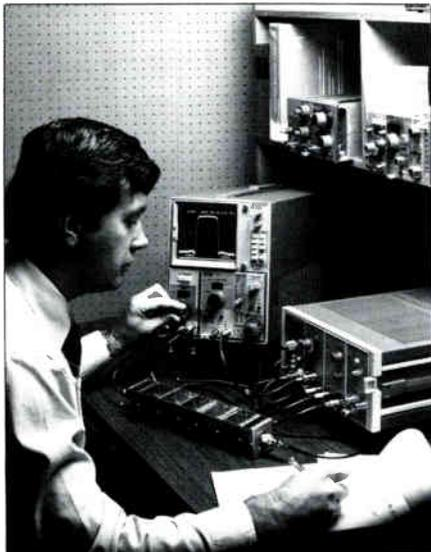
The model 7L14 spectrum analyzer from Tektronix, Inc.
