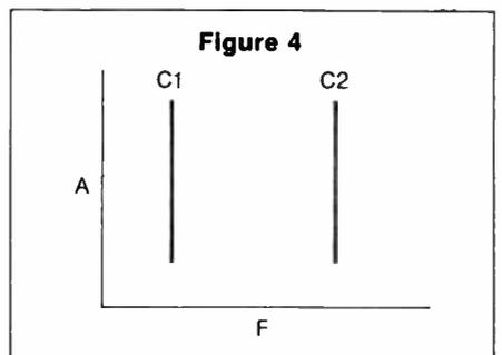
ard broadcast) radio works. Two signals mix together and produce a third signal which is different in frequency from the two original signals.
