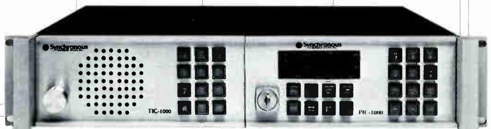
TIC-1000 and PIC-1000 modules pictured together in RMC-100 rack mountable chassis.
