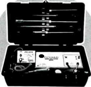
to detect the position of the fault along the conductor. The fault is located by the directional deflection of the receiver meter.
