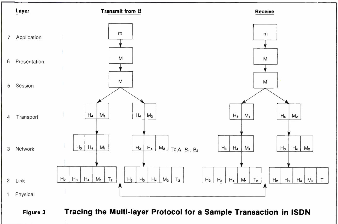
**Figure 3 Tracing the Multi-layer Protocol for a Sample Transaction in ISDN**
