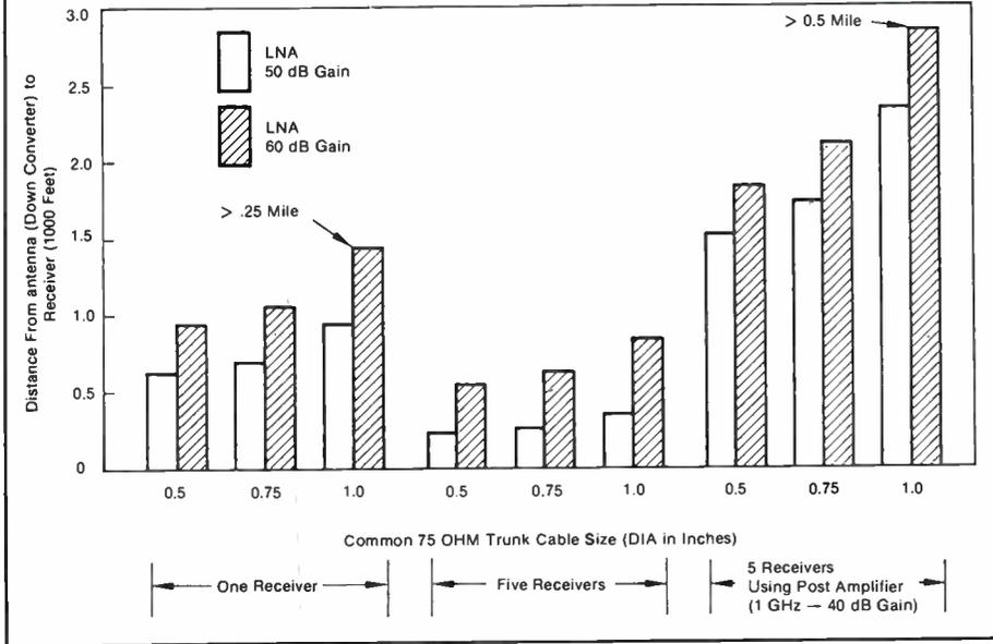
than a conventional 50 dB gain LNA) will extend the antenna/receiver distance more than one-half mile for some applications.
