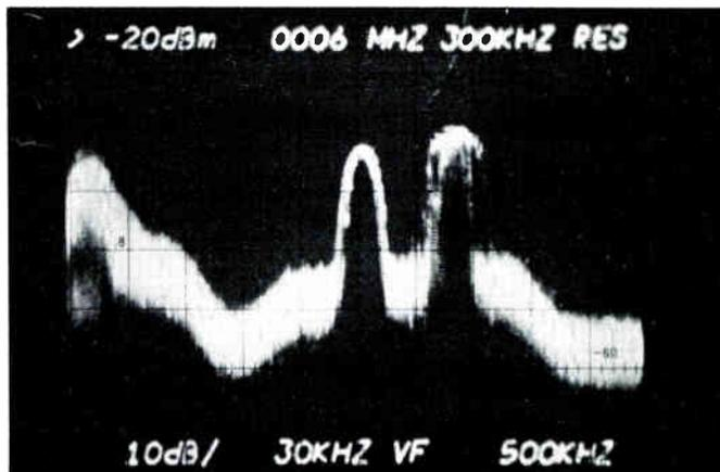
Figure 6a MTV Subcarrier Spectrum
