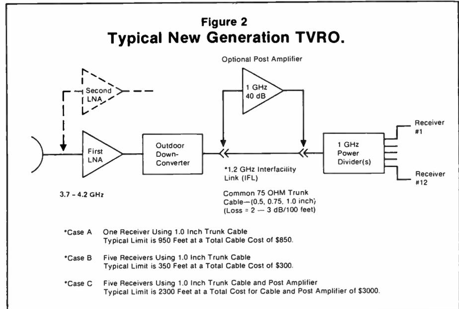
As indicated in Figure 1, the practical limit for distance between the antenna and receiver is somewhere between 400 - 800 feet. These relatively short distances place undue constraints on the antenna location site as well as cable operators pocketbooks. This 400 - 800 foot distance may not allow antenna positioning to take advantage of natural shielding (frequency coordinations) or
