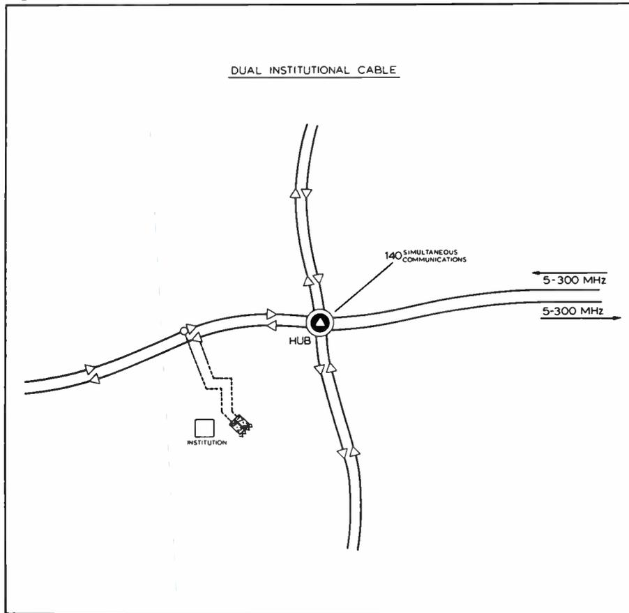
Multiplex Access / Collision Detection (CSMA/CO) philosophy and works on RF frequencies. All stations listen to the circuit. If the link is idle, the station requiring to transmit proceeds and listens for its own signal (echo) to confirm the transmission. Should two stations transmit simultaneously, the transmissions collide and each station attempts to retransmit after a random delay. 20 stations can be handled in a 300 KHz assignment, or 400 in a 6 MHz video channel.
