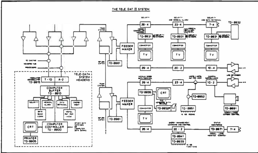
(Regional Interconnect) transmission. Data terminals talking to each other on the same system are coupled by an interlinking of two RS-232C ports. The front end computer is used for system status monitoring and billing records.
