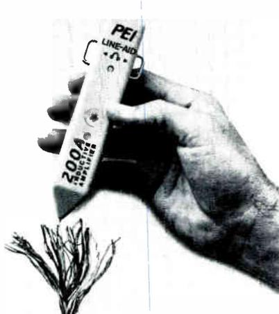
The 200A inductive amplifier is designed to identify and trace wires or cables within a group without damaging the insulation. The probe weighs 2 oz. and has a leather case. A tone from the probe's internal speaker indicates which wire is attached to the tone generating test set. A hand set can be clipped to the ears on either side of the probe if desired.
