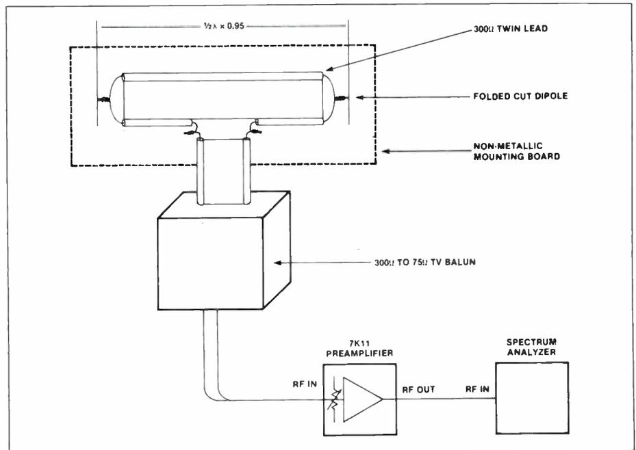
Figure 12-1 Details of homemade antenna and equipment connection for leakage measurements
