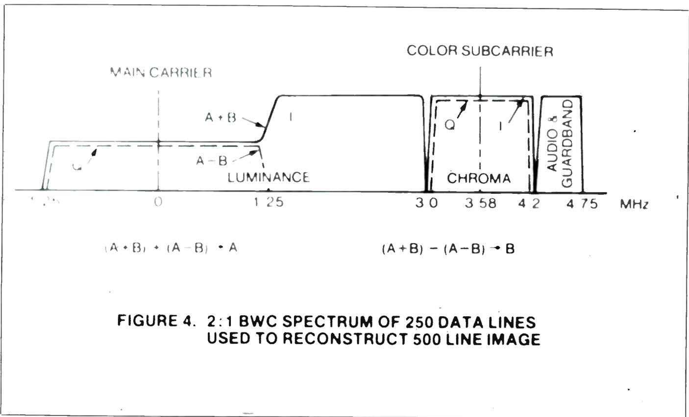
**FIGURE 4. 2:1 BWC SPECTRUM OF 250 DATA LINES USED TO RECONSTRUCT 500 LINE IMAGE**
