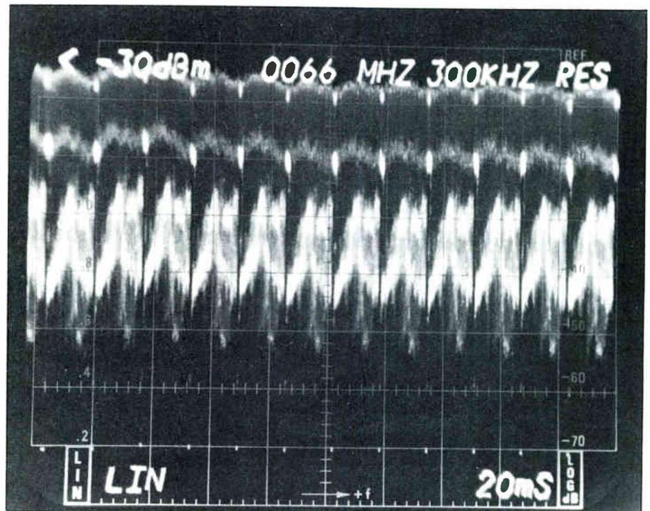
Figure 10-2 Measurement of hum and low frequency disturbance
