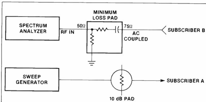
Figure 11-1 (left) Equipment connection for subscriber isolation measurement
