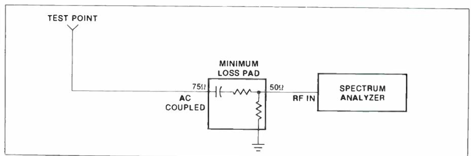
Figure 10-1 Equipment connection for hum measurements
