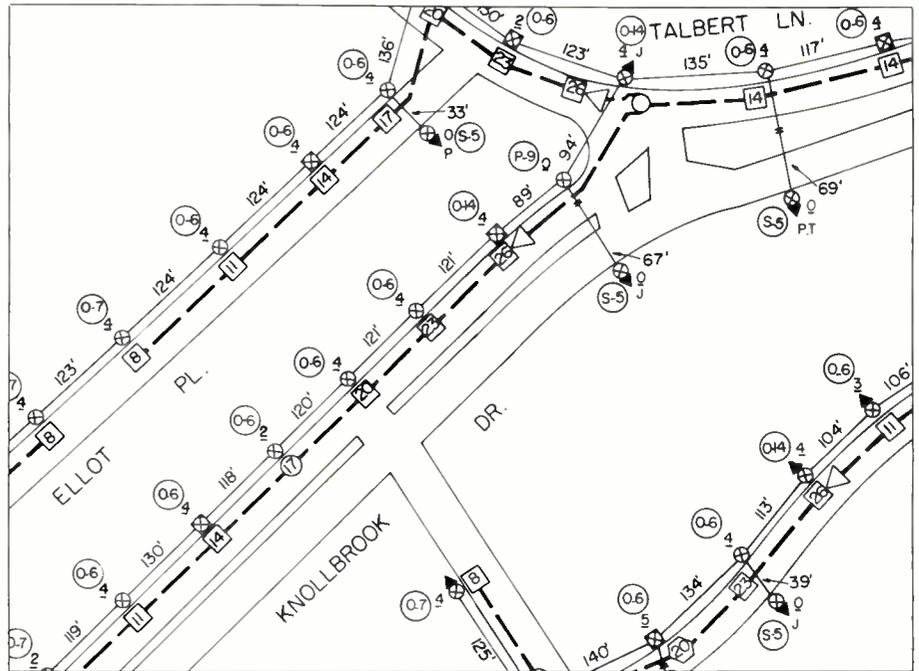
Figure 1 Strand map shows pole/pedestal locations marked with appropriate designations from a construction manual.
