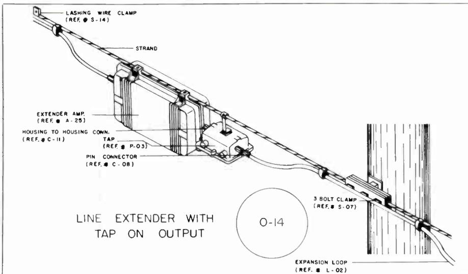
**Figure 2** This drawing from a construction manual illustrates the type of equipment and ancillary items required at a particular pole or pedestal location.
